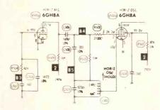
After the TV was brought to the shop, I checked the oscillator and phase-detector voltages. No dc voltage was measured at the plate of V501A (the AFC tube) and R509 checked open. Additional resistance measurements proved R514 and R533 were about 35% -low, while R507 measured only about 5K.
