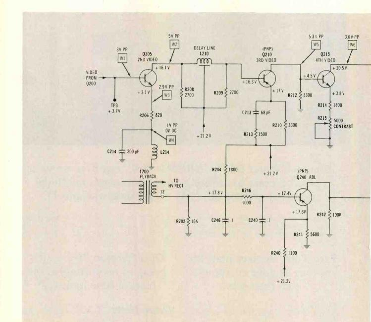
Figure 3 Three color matrixing power transistors and one video driver transistor with associated components are mounted on the picture tube socket module. All connections are made through polarized plugs and
