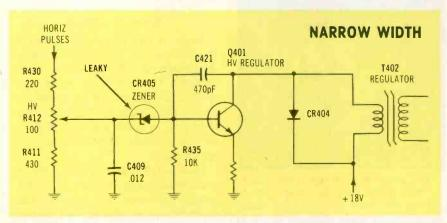
Figure 2 The narrow picture was caused by excessive HV-regulator operation. CR405 leakage forced Q401 to conduct too much saturation current through regulation transformer T402.
