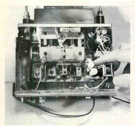
Figure 11 An ear-splitting shriek was the symptom of the 7985773 Delco radio. Filter capacitors often cause this trouble.
