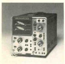
Maximum sensitivity of each vertical channel is 10 mV, and minimum sensitivity is 50 V per division. Bandwidth is from dc to above 15 MHz
