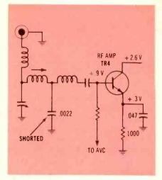
Figure 1 Audiovox model AMF-15 had no AM-band operation.
