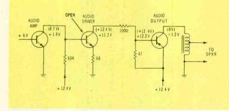
Figure 7 No click or thump could be heard when this inoperative Motorola TM7A was turned on. Usually a power problem or a dead output transistor is responsible.
