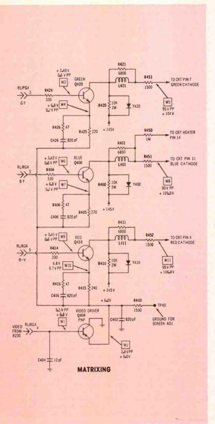
Figure 9 Luminance video and demodulated chroma signals are matrixed inside Q420, Q400 and Q410. Chroma signals are applied to the bases, and luminance signals are applied to the emitters. These four transistors are mounted on the CRT-socket module of Figure 3. Voltages and waveforms were measured during reception of a generator B&W signal, therefore, no chroma signals were there.
