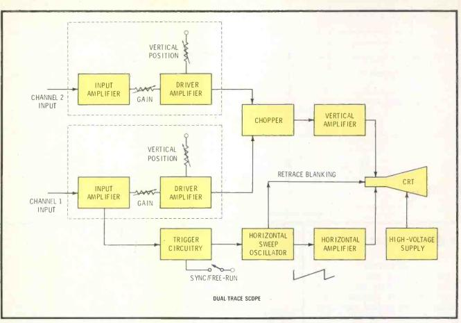
Figure 2 The block diagram of a service scope and a "bouncing-ball" medical scope are just alike. There are major differences of sweep speed, bandwidth and phosphor persistence.
