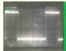
Figure 1 This good waveform (produced by a 30-MHz scope) has vertical leading and trailing edges (showing fast rise time), and sharp corners without ringing. (B) The same pulses on a 15-MHz scope have tilted leading and trailing edges (slower rise time), rounded corners with ringing, and no leading edge on the first pulse (it has no delay line).
