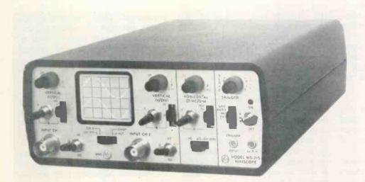
**Model MS-215** "Miniscope" from Non-Linear Systems operates for three hours on internal sealed lead-acid batteries requiring a charge. This dual-trace model has 10 mV vertical sensitivity and sweep times from 0.5 s/div to 0.1 µs/div.
