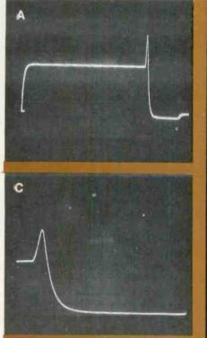
Figure 5 The full-time sweep magnifier often permits expansion without changing fifigger points, and gives better accuracy. (A) This is the pulse with the positive preshoot that's to be examined. (B) A faster sweep moves the preshoot off the screen, but rotating the Hickok multituin positioning control moves the magnified preshoot back to the screen. (C) The expanted pulse has been positioned for measurement of the duration.
