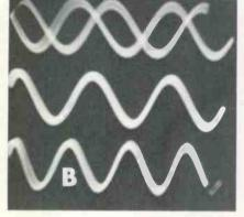
locking spot with two sine waves (bottom trace of A). Another CCW adjustment gives a false locking with two separate waveforms (top trace of B). Finally, more rotation of the frequency control results in three complete sine waves, as shown by the center trace of B. More sine waves may be obtained by additional CCW rotation (bottom trace of B).
