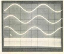
Figure 7 When the slope-polarity switch is in the "+" position, proper locking can be obtained at any point on the positive-going slope of a waveform except near the peaks. When the trigger-level control is turned to start the triggering too near
