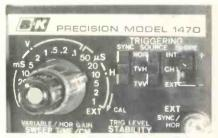
**Figure 9** In the B&K-Precision the "sweep-time/cm" switch supplies sweep between 100 ms and 1 *us*. The variable knob gives an uncalibrated but true increase of sweep time. In addition, a fixed X5 horizontal magnification can be switched in to give the effect of a 5-times decrease of sweep time. These are only two of the variations found in different models.
