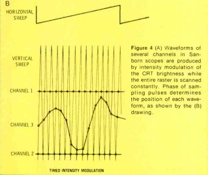
circuit, and the negative grid bias is decreased. Reduced negative grid bias allows the CRT to draw more gun current and produce a brighter trace.
