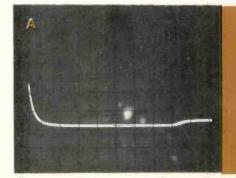
Figure 4 For examination of the trailing edges, triggering can be obtained from the positive preshoot that is there. (A) An ordinary scope without signal delay shows only part of the preshoot. (B) Wideband scope with signal delay shows all of the narrow preshoot so it can be measured.
