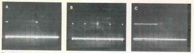
Figure 2 Using the simulated ignition-noise signal, this progression shows how pulse details can be revealed by shorter sweep times. (A) The pulses are stable, but appear blurred at 2 ms sweep. (B) A longer (slower)
