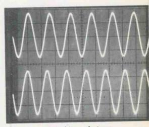
**Dual-trace** and dual-beam features allow two separate waveforms to be displayed at the same sweep speed. This is very useful for comparing the phase of signals and for fast troubleshooting of intermittents.
