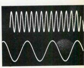
A 5X magnifier (expander) increases the horizontal sweep to 5 times screen width. Top trace is the sinewave signal needing magnification, while the bottom trace shows the same signal after the 5X switch is turned on. No other adjustments were made. This gives the effect of dividing the sweep time by 1/5 which spreads the waveform by a factor of 5.
