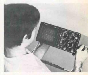
Ballantine model 1032A is a full-featured scope with a very unusual second triggering system that permits viewing two separate waveforms of different frequencies. Each dual-trace channel has its own Independent trigger circuit. Other features include 20-MHz response and an X10 magnifier.
