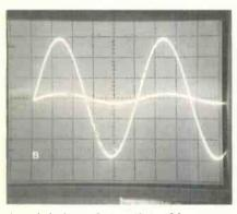
duced below that point. Of course, auto triggering showed an out-of-lock waveform. (B) However, when the triggering point was adjusted to the vertical center of this symmetrical waveform, a larger reduction of level did not disturb the triggering (locking).
