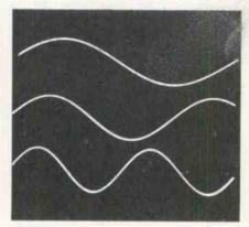
Figure 3 A triggered-sweep scope can be adjusted for any fraction of one cycle or almost any number of cycles. Within the range of the variable sweep-time control this change in the number of cycles is continuous. No relocking is required.
