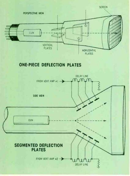
**Scope CRTs** have a reduction of deflection above certain high-frequency limits. It's caused by a phase change during the time the beam passes the large plate. One solution is to use several vertical plates and apply a successively delayed signal to each small plate in turn.
