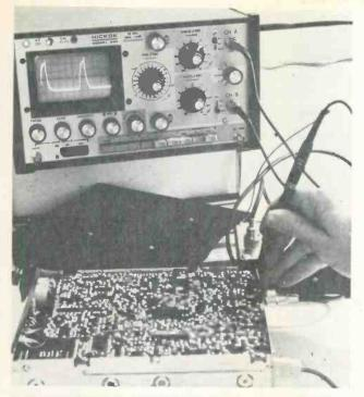
A communications technician is shown checking the noise-cancellation of a business-radio transceiver.
