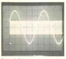
Figure 8 Triggering is not possible when the signal level drops below the voltage level selected by the triggerlevel control. (A) When the trigger level was about three-fourths up the slope, the triggering was eliminated when the signal amplitude was re-
