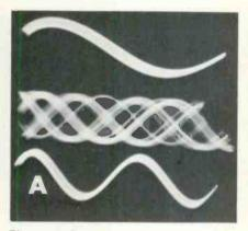
Figure 2 One limitation of recurrent scopes is that they can show only complete cycles, and relocking is required to obtain a different number. Beginning with a single sine wave (top trace of A), a CCW rotation of the frequency vernier to a lower frequency breaks the lock, and the waveform moves rapidly (center trace of A). Additional rotation locates another
