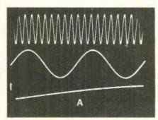
Figure 10 Changing the sweep time to give a different number of cycles does not affect the triggering (locking). (A) When two sine waves were triggered at the vertical center, the sweep time could be increased by 10 times (top) or decreased by 10 times (producing only a slope as shown at the bottom)
