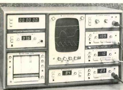
One rack holds a strip-chart recorder, two blood-pressure monitors, cardio amplifier, respiration monitor, temperature module, cardio-rate module, a timer and a four-channel scope. Similar monitors are used in intensive-care units (ICU) and operating rooms.
