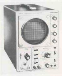
Vertical sensitivity of 10 mV/cm and triggered sweep from 0.5 s/cm to 0.5  $\mu$ s/cm are some specifications of the workhorse Simpson model 455T single-sweep scope.
