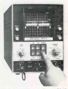
Six pushbuttons on the Sencore PS-29 "Minute Man" panel select the sweep times most often needed. Also included Is the usual time/cm switch with frequency markings. Locking is automatic without any variable controls.
