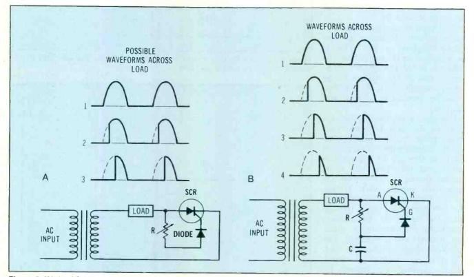
Figure 5 (A) An SCR that's gated by ac controls power to load. Waveform 1 is half-cycle, 2 is less than half-cycle, 3 is quarter-cycle of applied current. This circuit is limited to a control range between ½ and ¼ (90°) of cycle. In B, adding a capacitor allows control over the entire half-cycle (180°).
