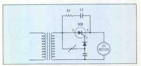
Figure 6 In some speed controls, the motor might be connected in the cathode circuit of the SCR. R1 and C1 prevent self-triggering of the SCR due to inductive-load kickbacks.
