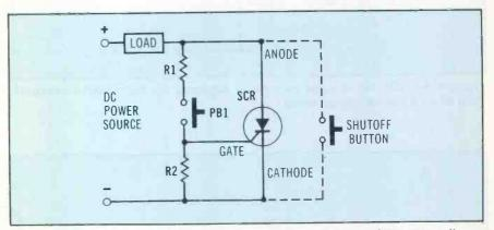
Figure 2 SCR in a dc circuit does not conduct until gate voltage turns it on, despite forward cathode-anode bias.
