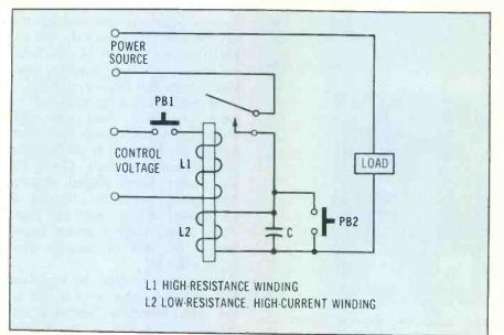
Figure 1 An SCR may be compared to a current-locking relay that stays on after being activated, then unlatches when the hold-in coil is shorted out.
