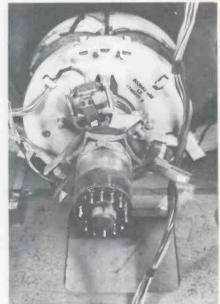
The convergence-yoke assembly was crooked on the picture-tube neck, evidence of previous poor servicing.
