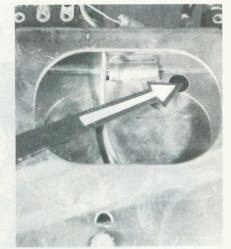
Many of the older tuners with Nuvistor RF amplifiers by now have had tuner cleaners sprayed accidentally into the neutralization trimmers. This gives the effect of wrong neutralization and produces oscillation on some highband channels. The trimmers must be thoroughly cleaned out with a solvent and allowed to dry before they are adjusted.
