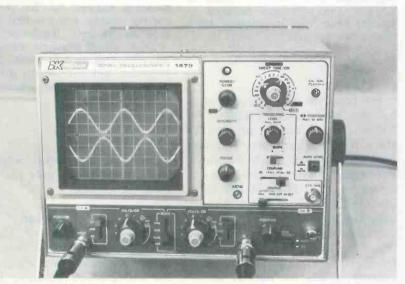
**B&K-Precision model 1479** is a new wide-band oscilloscope with many features making it an indispensable instrument for all types of service work.
