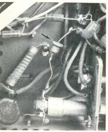
Another servicing mistake was the conventional *top-hat* diode used as a boosted-boost diode. This one was not shorted, but it should have been, for these are called on to supply about 300V of extra dc voltage—far above the ratings of the wrong replacement.
