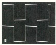
Figure 2 (A) Each channel has a lever-type ac/dc coupling switch that is convenient to operate. (B) Square waves of 20Hz had no tilt during dc-coupling operation. With the lowcapacitance probe and ac coupling, the tilt at 20Hz is barely noticeable (bottom trace, indicating good low frequency response.
