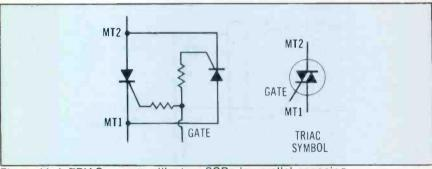
Figure 11 A TRIAC operates like two SCRs in parallel-opposing.
