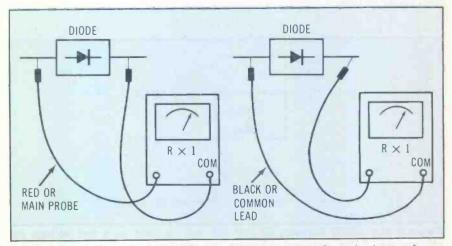
Figure 7 Use a diode to reveal polarity of voltage coming from the leads of your ohmmeter.
