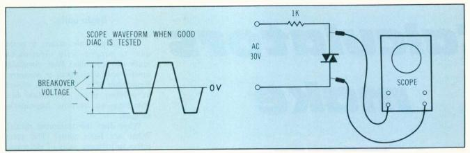
Figure 15 DIAC testing with ac and oscilloscope may not reveal imbalances, unless dc scope coupling is used.
