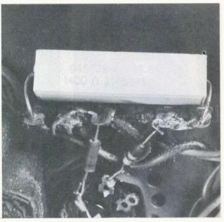
Heat from the large 20W 1400  $\Omega$  wire-wound resistor deteriorated all soldering joints on the terminal strip and carbonized the insulation. None of the joints were open, but would have gotten worse with time.
