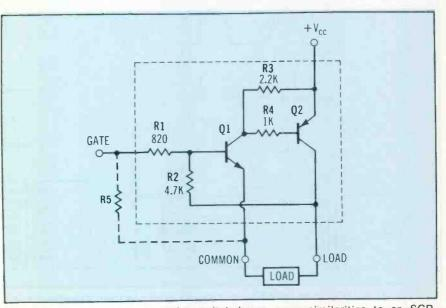
Figure 3 A transistor regenerative switch bears many similarities to an SCR. Resistors' values are typical for Vcc of 6V to 12V.
