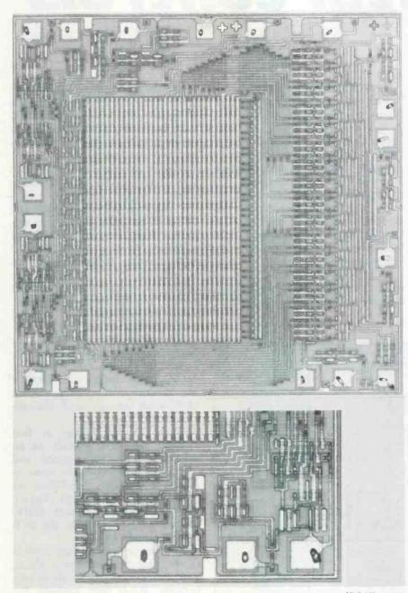
For the Motorola model MCM1452 1024-bit Read-Only Memory (ROM), one picture shows the entire IC chip, which is about a quarter-inch square. The other is a 27-times enlargement of one corner of the same chip. (Courtesy of Motorola)
