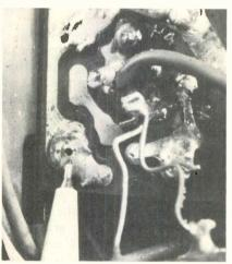
A pen points to the hole in a ground joint of the IF board where a ground lance had pulled loose. Erratic color level often results from opens at auxiliary grounds.
