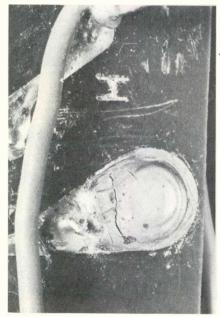
This crack at a ground in the oscillator circuit extended around the rivet completely. It caused intermittent operation of the horizontal oscillator. Flexing of the board made the crack more visible.
