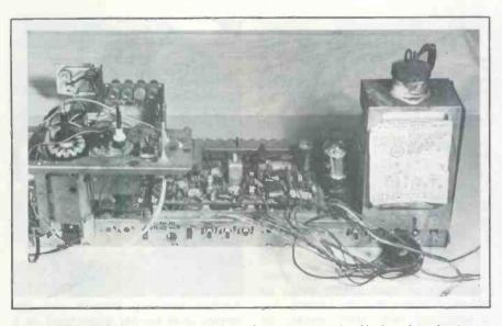
An old RCA CTC16 chassis was selected as an example. Notice that the tuner assembly is mounted correctly on the chassis for servicing or transportation. Two chassis screws and matching slots in the tuner bracket hold the assembly. (If the tuner is placed on top of chassis wiring severe damage can occur to unshielded coils and other fragile components.)
