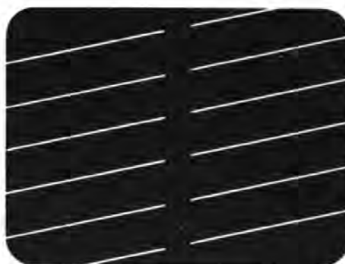
Fig. 7-6. Proper slant of vertical-retrace lines.
