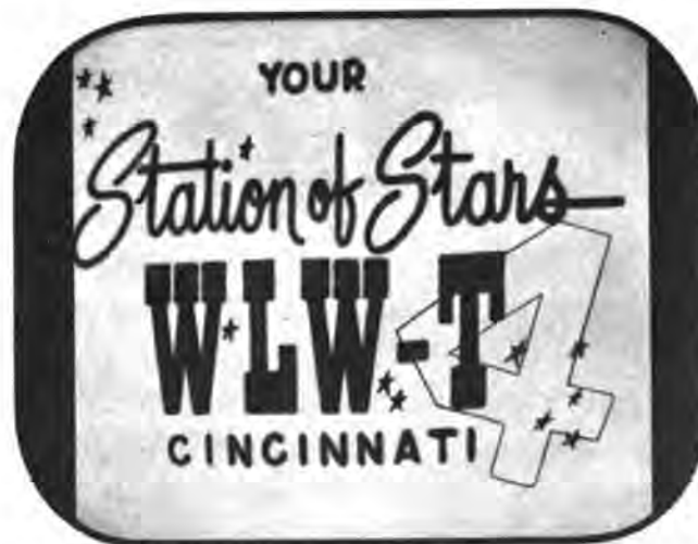
Fig. 1-7. Lack of adequate width in picture. Courtesy Crosley Corp.
