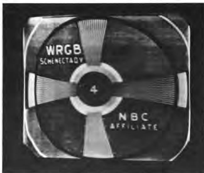
Fig. 4-7. Poor horizontal linearity, with right side of picture stretched excessively. Courtesy General Electric Co.
