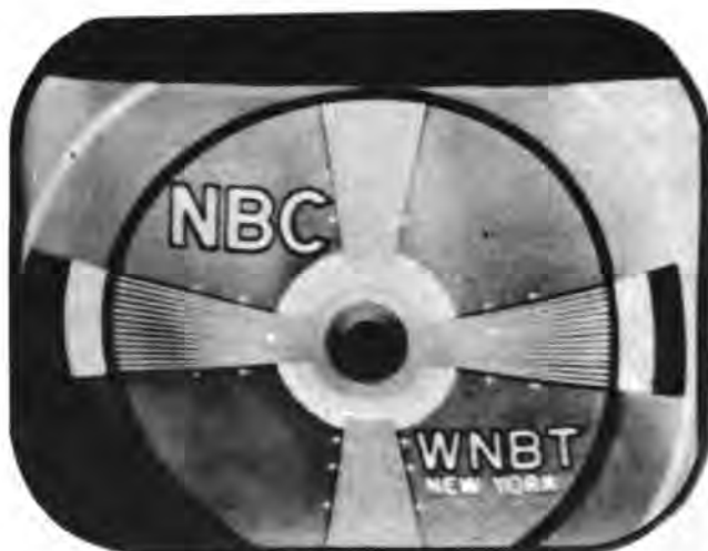
Fig. 7-10. Picture showing neck shadow. Courtesy RCA Service Co.
