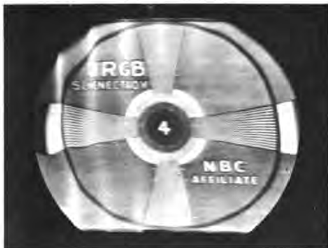
Fig. 1-6. Picture showing cross-talk of the horizontal-sweep frequency components into the vertical-deflection coils. Courtesy General Electric Co.
