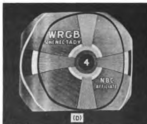
Fig. 2-1. (A) Typical horizontal-output section of a tv receiver. After Admiral Corp. (B) Reduced width, compressed left side. Courtesy RCA Service Co. (C) Reduced width, foldover at right. (D) Reduced width, compressed right side. Courtesy General Electric Co.
