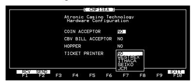
This routine allows to configuration of the machine according to the actual installed hardware like coin and bill acceptor, hopper and ticket printer.
