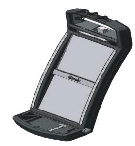
7. Lift the front part of the playfield frame and carefully pull the cables through the opening of the back part of the playfield frame.
