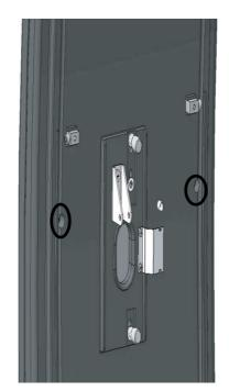
5. Remove the two screws at the bottom of the playfield
