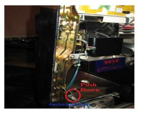
It will feel pointed, so using your fingers pull down on this point, and the door will open. If this is not working for you, you can lay the machine on it's left side, and do the same procedure.
