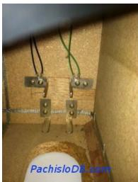
Some games still have the probes installed, if these become shorted, they can cause an OF error do be displayed and an alarm to sound when playing the game. To keep this from happening anymore, turn off the game, locate the probe's and wires on the bottom right of the game, to the right of the hopper.
