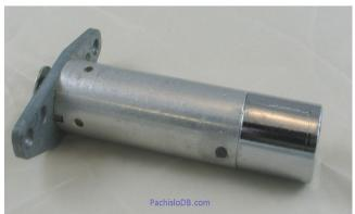
The picture above shows the re- assembled lock and cylinder Epoxy was used to fill the holes to keep the cylinder and the lock together. What ever you use to keep these parts together, it can't protrude past the edges of the lock or it will not fit into the door for mounting. You can also use an ink pen cartridge to put in place of the pins that had to be drilled out, securing them with some super glue. Just make sure that the fit is a bit tight to start with, if it's
