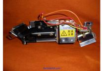
The mech pictured above, you should see the bottom of the track with out even removing the mech from the door. Others may have screws that need to be removed before you can remove them from the door.
