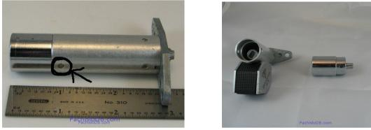
Step one: You will need to drill out the pins that hole the cylinder in the lock assembly. You may want to start with a very small drill to put a small divot in the pin's center to have a good starting point for the larger drill bit, or you can use a nail or very small center punch with a point.
