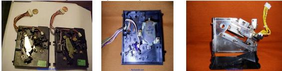
The unit's pictured just above are able to be removed easily from the door, you simply need to find the clip usually on the Left side, pull the clip away and pull out the mech, it should come right out.
