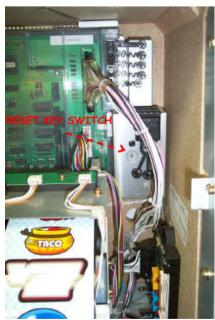
Or on newer machines such as TACO SLOT and BABEL, the reset key switch is to the right of the reels as pictured above right.
