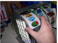
Now that the screws are removed, and the connectors are pulled from the sockets, grasp the reel assembly and pull forward. It should come right out. If something is getting hung up look for a screw or connector got missed.
