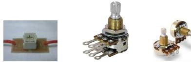
These are installed in the game, by cutting one side of the speaker wire, and using the center and the right side taps on the "POT" or Potentiometer. The type pictured center and to the right, above need to have the leads soldered to them. Where as the type pictured on the left have leads already to connect using small "Butt" connectors that are crimped on to bare ended wires of the speakers.
