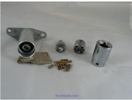
Once the pin's have been drilled out, the cylinder will come out of the lock assembly as pictured Left.
