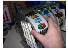
Now that the screws are removed, and the connectors are pulled from the sockets, grasp the reel assembly and pull forward. It should come right out. If something is getting hung up look for a screw or wire connectors that got missed.
