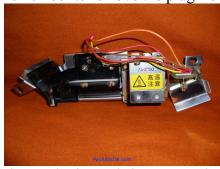
The mech pictured above, you should see the bottom of the track with out even removing the mech from the door. Others may have screws that need to be removed before you can remove them from the door. Like the one pictured above. Make note of how the angle of yours looks before you do these types, so you can re-install them properly.
