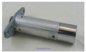
The picture above shows the re- assembled lock and cylinder Epoxy was used to fill the holes to keep the cylinder and the lock together. What ever you use to keep these parts together, it can't protrude past the edges of the lock or it will not fit into the door for mounting.
