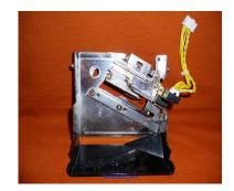
The unit's pictured just above are able to be removed easily from the door, you simply need to find the clip usually on the Left side, pull the clip away and pull out the mech, it should come right out. Remember to remove the plug from the connector when removing the coin mech.
