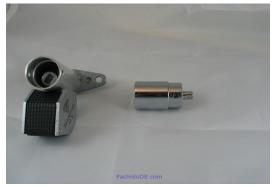
Step one: You will need to drill out the pins that hole the cylinder in the lock assembly. You may want to start with a very small drill to put a small divot in the pin's center to have a good starting
