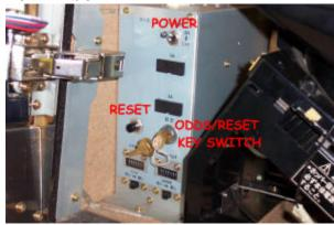
or on newer machines such as TACO SLOT and BABEL, the reset key switch is to the right of the reels:
