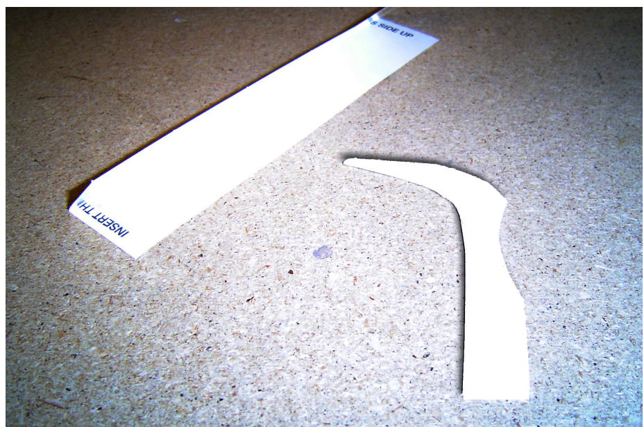
Figure 3. - Makeshift removal tools for removing coins from card slot without damaging the optic mechanism.
