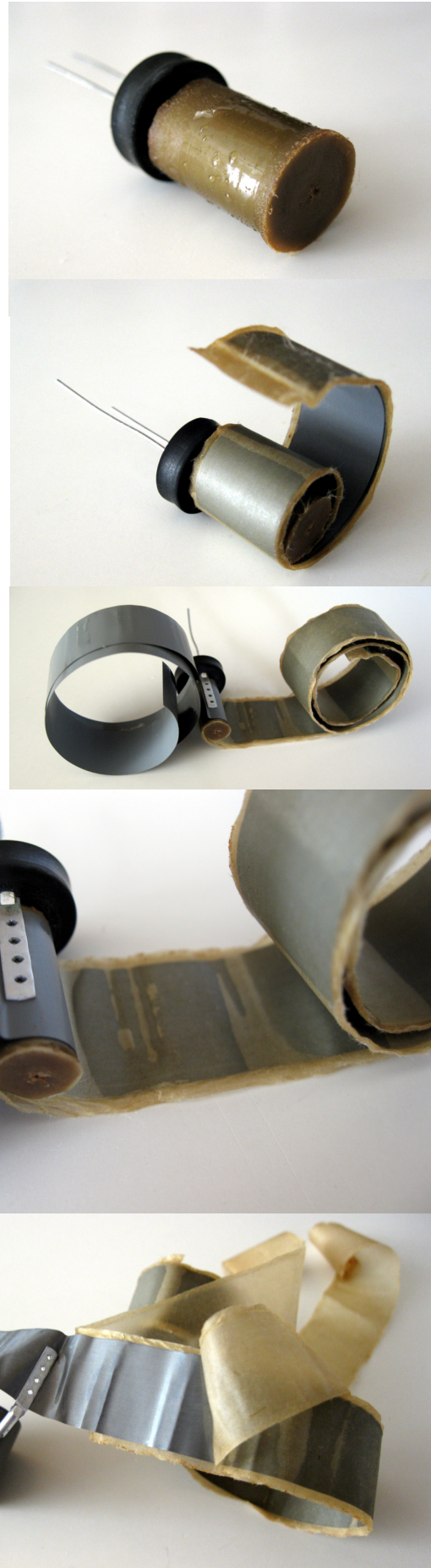
From top to bottom, this is what's inside an electrolytic capacitor. It's two strips of aluminum foil, separated by two strips of paper (soaked in liquid electrolyte) and rolled up. You can see that it's quite wet. When the electrolyte dries out, the capacitor's ESR increases causing problems.
