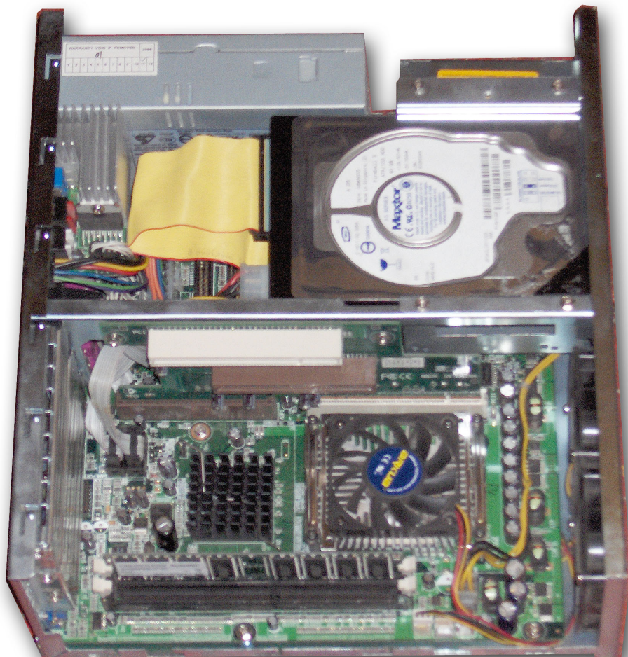
Motherboard cleaned and capacitors replaced
