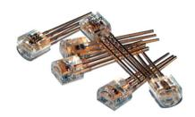
All diodes and transistors react to light to some degree. When electromagnetic radiation hits the junction region, it causes minority current carriers in the diode, making the diode conduct slightly. To make a phototransistor more sensitive to light, all we had to do was redesign the physical makeup so light can get to a photo diode between the base and collector of a transistor. The light hits the diode and starts the diode con-
