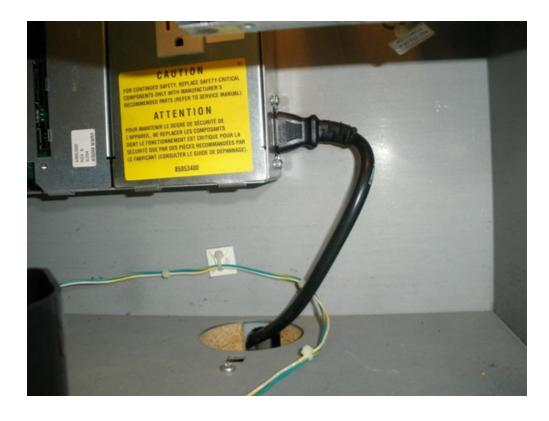
Place the hopper back into the slot machine making sure it slides in easily and completely with the base rails on hopper guides on the bottom of the machine. The hopper plugs into a receptacle toward the back of the machine. It is designed to fit in easily without using excessive force.
