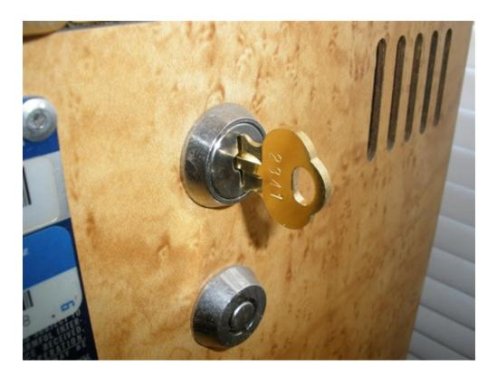
Insert the Jackpot Reset Key into the keyhole. Turn the key ONLY ONE-QUARTER TURN TO THE RIGHT! This will reset the machine, and once you close the main slot machine door, you will be ready to resume play.
