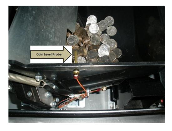
Provided your slot machine sets on a regular casino slot machine stand with holes in the top and the holes are aligned with the slot machine, those coins which bypassed the hopper will go down the chute, through the hole in the bottom of the machine, through the hole in the top of the stand, and into the open area in the stand cabinet.
