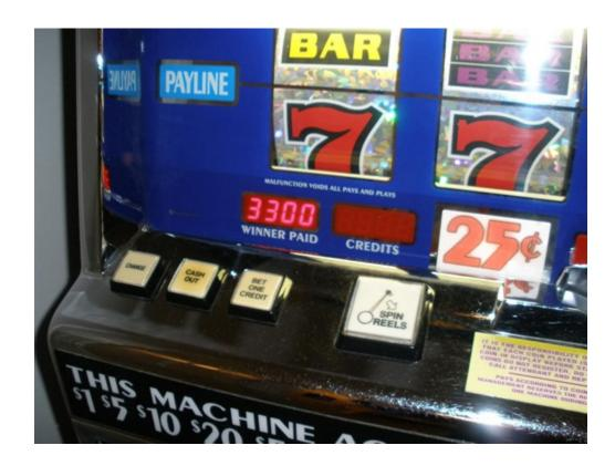
Open the main slot machine door. Look into the hopper. If it is empty or has just a few coins or tokens, place about 500 coins or tokens back into the hopper. Close the main slot machine door. In a few moments you should hear the sound of the hopper's motor turning and soon the remaining coin payout will begin.
