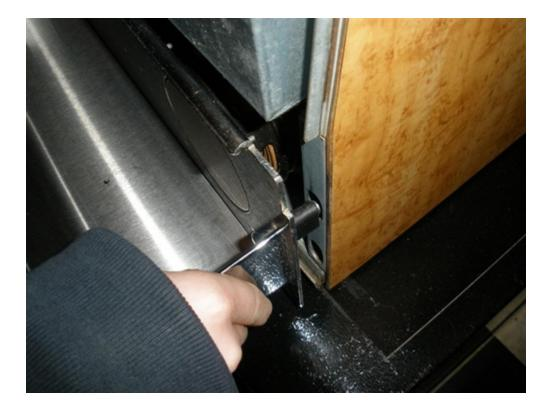
The hopper is on the bottom floor of the machine and slides out on two base rails along two metal guides. Slide the hopper out slowly by grasping the handle with your left hand and supporting the hopper with your right hand. Do not use the black hopper bowl to pull the hopper out of the slot machine.
