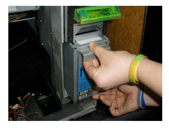
Hold the cash box in both hands and turn it upside down. Notice on the bottom of the cash box is a door which has two small finger sized holes on one side. Normally the door is held closed by a small piece of electrical tape so the bottom cash box door doesn't come open while removing it from the cash box chassis of the slot machine.
