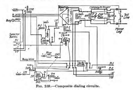
apparatus. At the left center are the selector banks by means of which the toll line can be called automatically. This is used if this is a toll switching office as described under the head "Toll Switching Office." In the upper right-hand corner is the toll line with the composite ringing 20 apparatus. The rest of the apparatus is a selector which has access to the automatic exchange or may form part of it.
