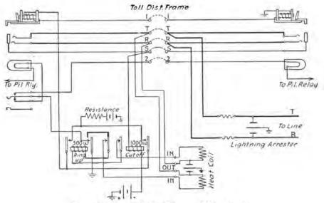
FIG. 242 .- A typical toll or rural-line circuit.
