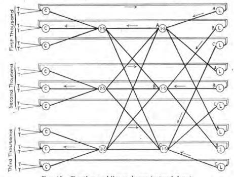
FIG. 15.—Ten-thousand-line exchange (network form).
