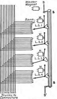
FIG. 43.—Scheme of master-switch control of Keith lineswitches.
