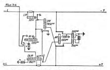
FIG. 72 .- Trunk holder with parallel battery feed.
