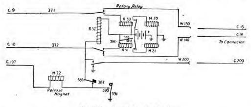
FIG. 228.-Second selector circuit.
