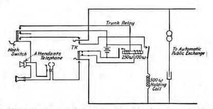
FIG. 154.-Trunk circuit to attendant's station of a push-key inter-communicating system.
