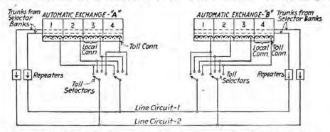
FIG. 268.-Two community automatic exchanges with free automatic trunks.
