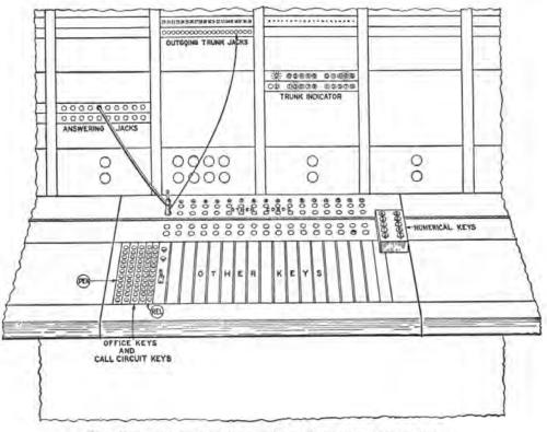
FIG. 219.-Manual position with push-button calling device.
