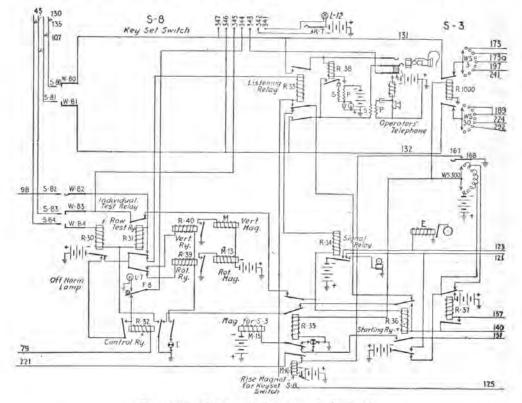
FIG. 225 .- Operator's keyset switch circuit.
