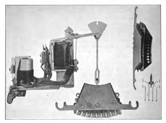
FIG. 44.-Keith lineswitch with an unwired bank.
