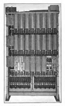
FIG. 90.-One-hundred-line switchboard, rotary lineswitches (back).
