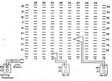
FIG. 1.-Essential principle of connector switch.
