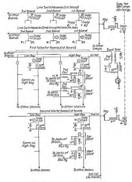
FIG. 290.-Selector and connector supervisory scheme.
