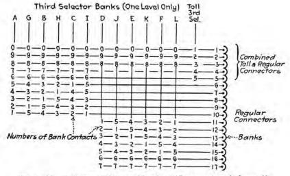
FIG. 138.—Selectors (3'd) trunking into 17 connectors (scheme 1).
