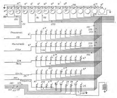
FIG. 227.-Sending machine and keyset circuit.
