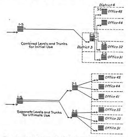
FIG. 142.-Trunking, inter-office, two levels combined for initial service.
