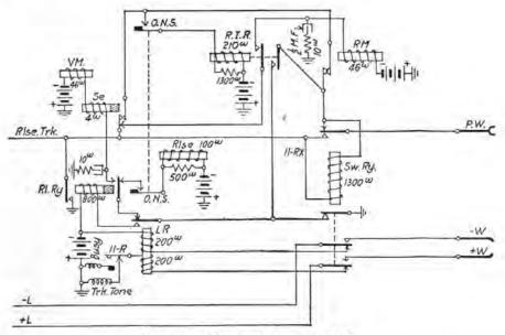
FIG. 63.-Circuit of selector switch.
