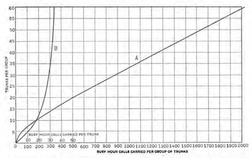
FIG. 305.—Curve A shows call-carrying capacities of trunk groups of various sizes between automatic central offices; average trunk holding time of 83 seconds. Curve Bshows call-carrying capacity of each trunk in groups of various sizes.
