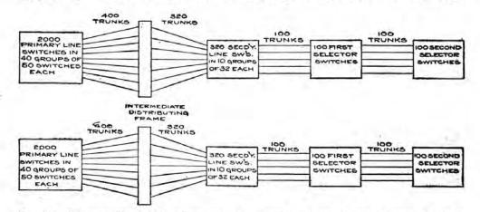
FIG. 77.—Diagram illustrating scheme of using secondary lineswitches to reduce first and second selectors.
