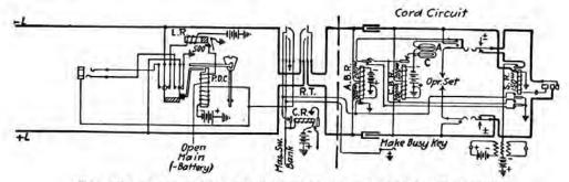
FIG. 194.-Automatic traffic distributor, lineswitch and cord circuit.
