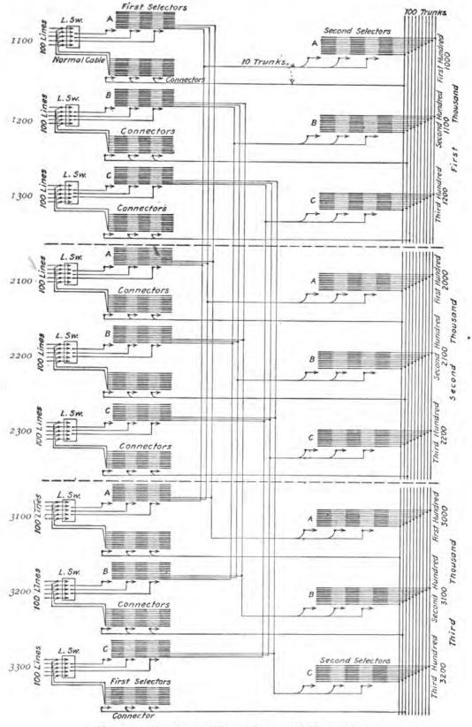
FIG. 16 .- Ten-thousand-line exchange with lineswitches,
