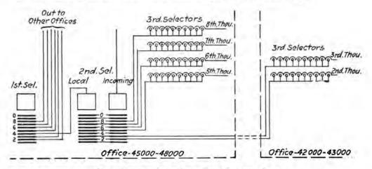
FIG. 22.—One first-selector level for two offices.
