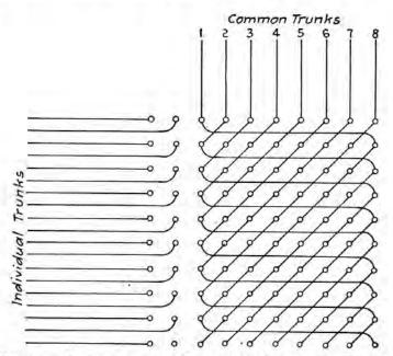
FIG. 126 .- Common trunks added to individual trunks, ELS-15.
