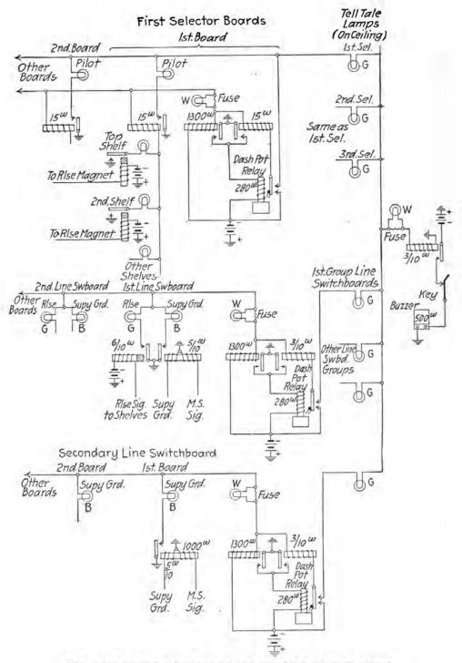
FIG. 289.-Release signal supervision, tell-tale and alarm scheme.
