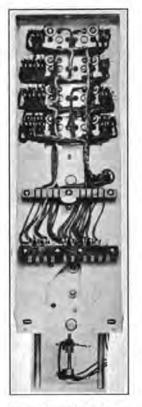
FIG. 51.—Automatic relay mounting, top view.
