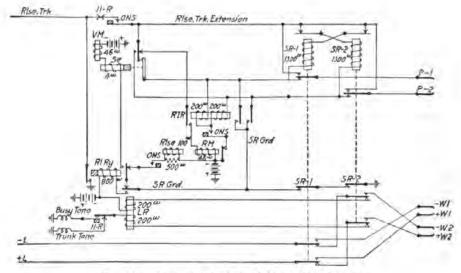
FIG. 64 .- Circuit of 10-level 20-trunk selector.
