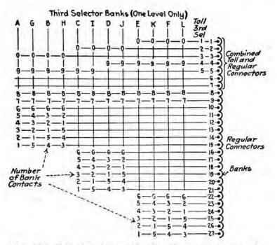
FIG. 140.-Selectors (3'd) trunking into 27 connectors (scheme).
