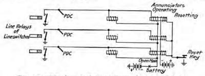
FIG. 163.-Watchman's clock and annunciator connections.
