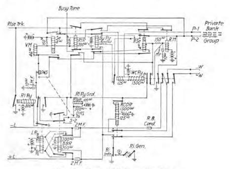
FIG. 84.-Circuit of 2-digit group connector.
