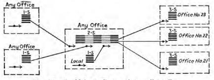
FIG. 29.—Combining traffic at an intermediate office.
