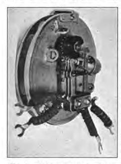
FIG. 39.—Automatic telephone calling device.
