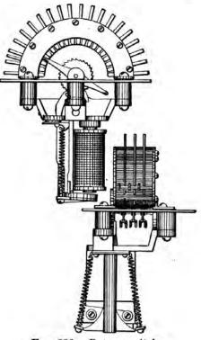
FIG. 236.-Rotary switch.
