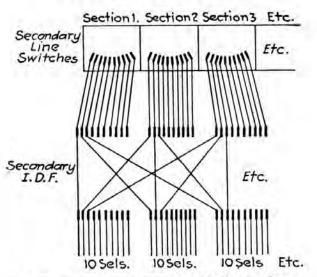
FIG. 96.—Secondary intermediate distributing frame.
