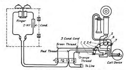
FIG. 147.-Desk telephone wiring diagram.
