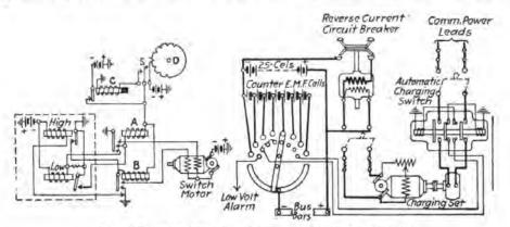
FIG. 274.—Automatic voltage regulation for C.A.X.
