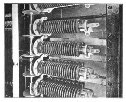
FIG. 214.—Sequence switches mounted.
