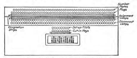
FIG. 278.-Diagram of keyshelf with call indicator.
