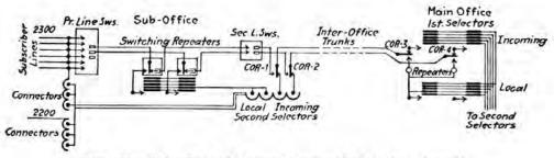
FIG. 35.-Sub-office with 2-way trunks and switching repeater.
