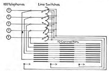
FIG. 8.—One-hundred-line system with rotary lineswitches.
