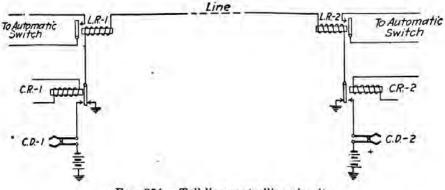
FIG. 254.-Toll line controlling circuit.
