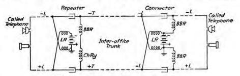
FIG. 69.-Talking circuit of an inter-office connection.
