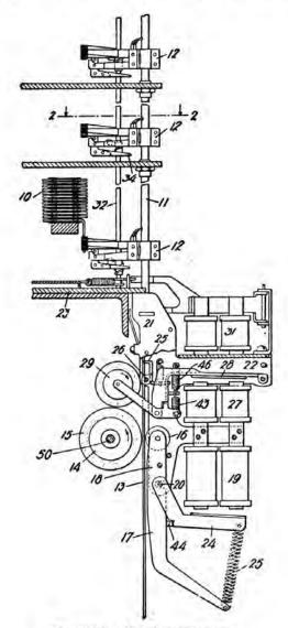
FIG. 212.-Clutch mechanism.
