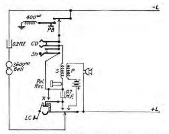
FIG. 261.-Local battery automatic telephone circuit.
