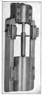
FIG. 281.—Solenoid ringing current interrupter.
