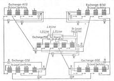
FIG. 271.-Typical network of community automatic exchanges.
