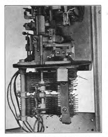
FIG. 66.-Vertical wiper and bank, operated.
