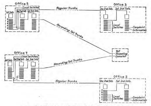
FIG. 143.-Trunking, recording toll and miscellaneous service.
