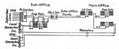
Fro. 34.—Sub-office with switching repeater, 10,000-line system switch on second digit.
