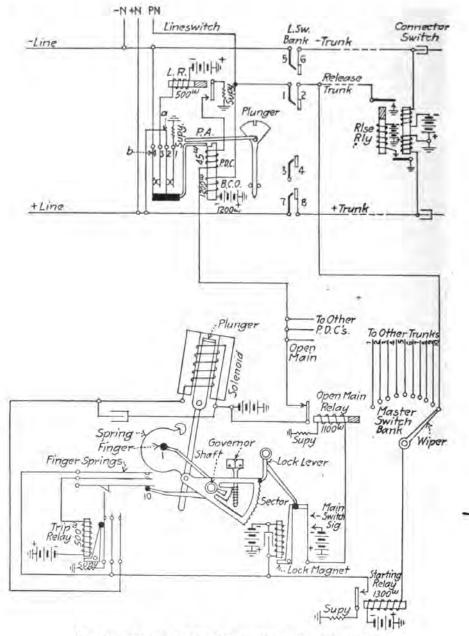
FIG. 46.-Circuit of Keith lineswitch and master switch.
