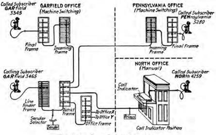
FIG. 202.-General plan of trunking.
