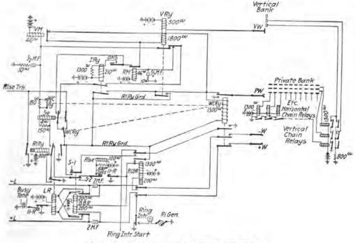
FIG. 85.—Circuit of 1-digit group connector.
