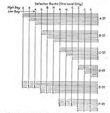
FIG 134.—Selector trunking (one level). Sections grouped by 3's and 6's.
