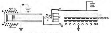
FIG. 191.-Diagram of circuit of Christensen pneumatic selector.
