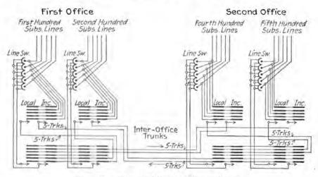
FIG. 18.-Thousand-line, 2-office exchange.
