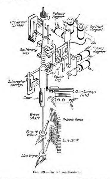
When the subscriber dials the first digit of the call number, the linerelay armature vibrates one complete cycle for each unit in the digit. Thus it feeds current alternately to the release relay and to the vertical magnet. The former is slow release, and remains energized throughout the series of pulsations which it receives. The vertical magnet is quickacting, follows the impulses and lifts the wiper shaft. The series relay Se
