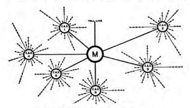
FIG. 269.-Radial system of exchanges.
