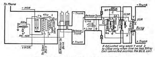
FIG. 168.—Discriminating outgoing trunk circuit.
