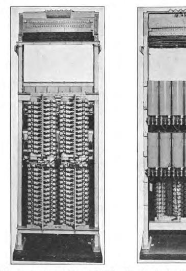
Fig. 86.—One-hundred-line switchboard, Keith lineswitches (front).
