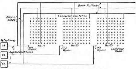
FIG. 2.-Principle of 100-line exchange.
