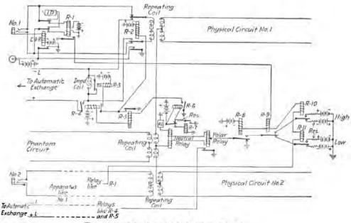
FIG. 257.-Quadruplex dialing on toll lines.
