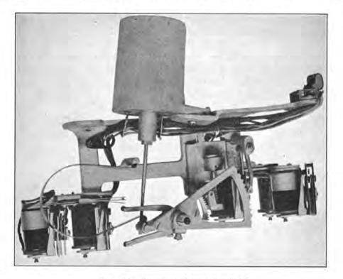
FIG. 47 .- Unmounted master switch."
