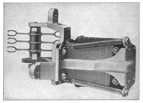
FIG. 235.—Wipers and magnet of rotary switch.
