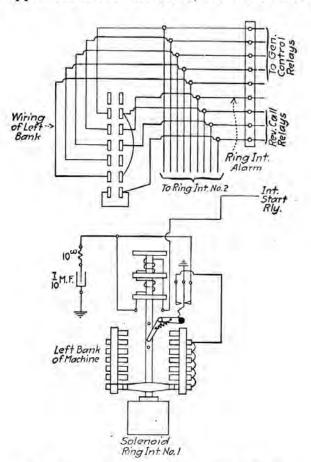
FIG. 288.-Solenoid ringing interrupter circuit.
