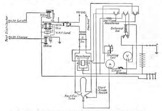
FIG. 285.—Circuits of a mercury arc rectifier charging outfit for a sub-office.
