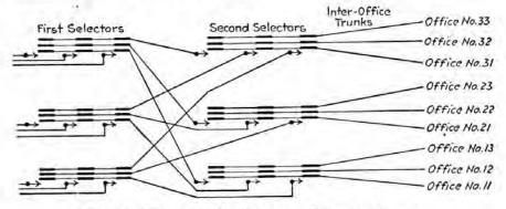
FIG. 25.—Direct trunks with first and second selectors.
