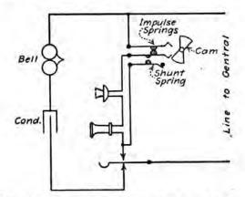
FIG. 41.-Automatic telephone circuit, series type.
