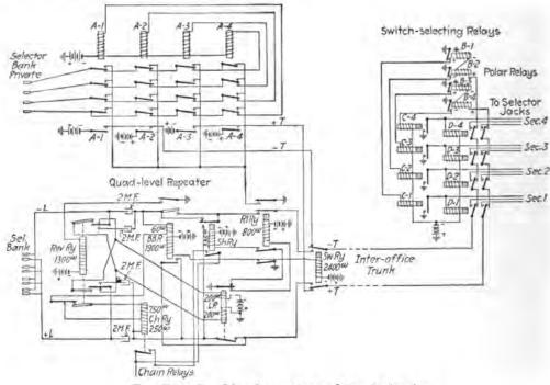
FIG. 75.-Quad-level repeater and trunk circuits.
