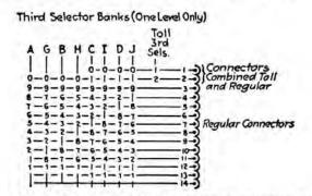
FIG. 136 .- Selectors (3'd) trunking into 14 switches (scheme).
