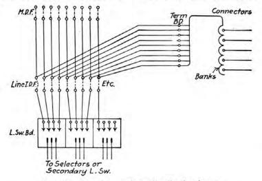
FIG. 91.—Line intermediate distributing frame.
