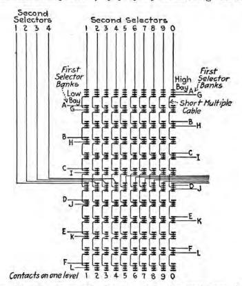
FIG. 129.-Selectors trunking into 14 switches (terminal connections).
