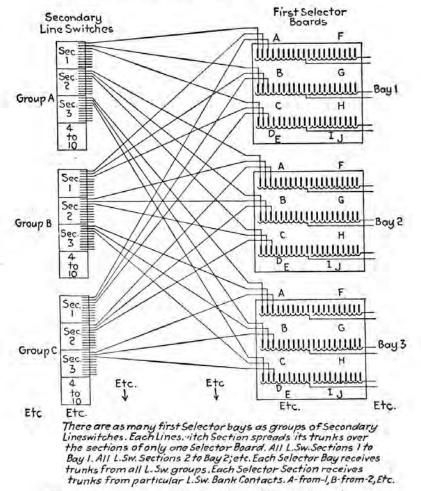
FIG. 97.-Trunking secondary lineswitches to first selectors.
