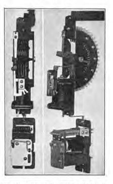
cut-off relay, drawing current through the magnet and springs 3-4 of the line relay, pulls up, switching both subscriber lines -L + L from ground, line relay and battery to the wipers -W + W. It also switches the private wiper PW from the test circuit of springs 1-2 of the line relay LR to the private normal and the cut-off relay.
