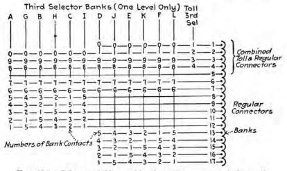
Fig. 139.-Selectors (3'd) trunking into 17 connectors (scheme 2).
