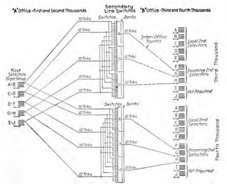
FIG. 20.—Outgoing secondary lineswitches, 10,000-line, 2-office exchange.
