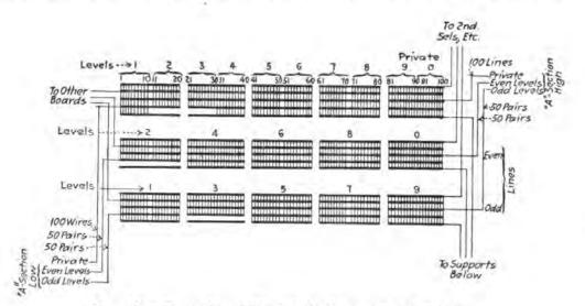
FIG. 106.-Expansion of Fig. 105 showing separate terminals.
