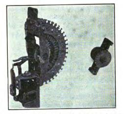
FIG. 205.-Rotary switch for sender selector.
