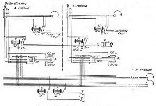
FIG. 192.-Circuit of automatic order wire system.
