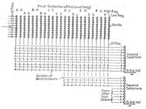
FIG. 128.-Selectors trunking into 14 switches (scheme).
