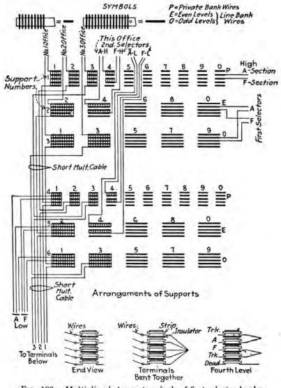
FIG. 103.-Multipling between terminals of first-selector banks.
