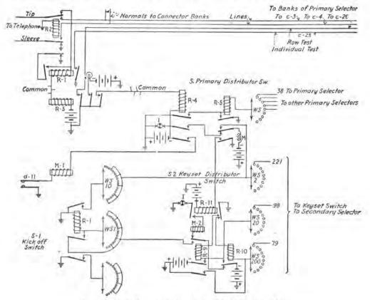
FIG. 222.—Subscriber's line and distributor circuits.
