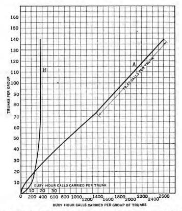
FIG. 304.—Curve A shows call-carrying capacities of trunk groups of various sizes, manual central offices; average trunk holding time of 120 seconds. Curve B shows call-carrying capacity of each trunk in groups of various sizes.
