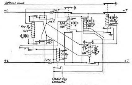
FIG. 67.-Circuit of impulse repeater.
