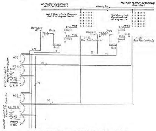
FIG. 223.-Relation between distributors and keyset switches.
