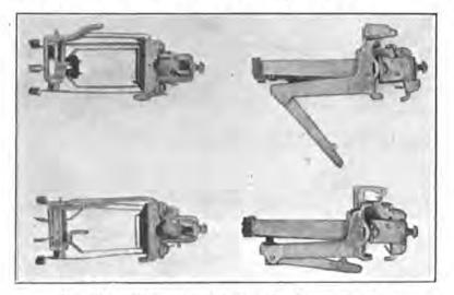
FIG. 210.-Selector brush, operated and non-operated.
