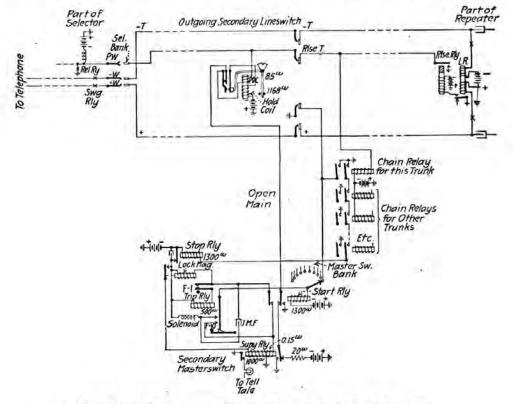
FIG. 79.-Circuit of outgoing secondary lineswitch, Keith type.
