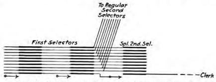
FIG. 127.-Special second selectors to care for preliminary impulse.
