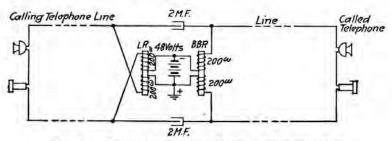
FIG. 61.-Talking conditions in single-office exchange.
