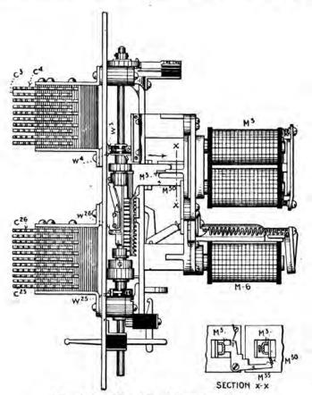
FIG. 239.-Side view of 2-motion switch.
