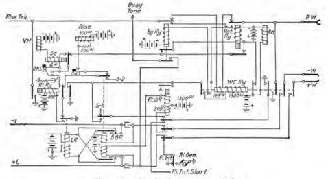
FIG. 60.-Circuit of connector switch.
