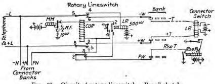
FIG. 49.-Circuit of rotary lineswitch. Pencil sketch.
