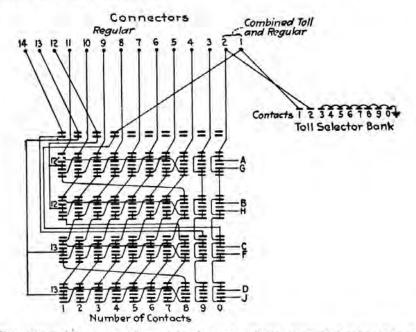
Fra. 137.-Selectors (3'd) trunking into 14 switches (terminal connections).
