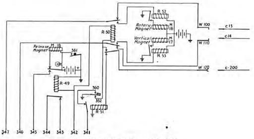
FIG. 232.-Selector for reverting calls.
