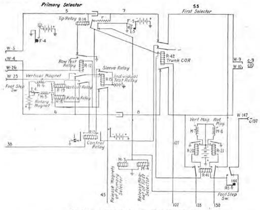
FIG. 224.-Primary and first selector circuits.
