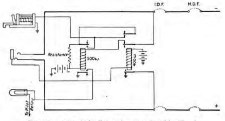
FIG. 246.-A pay-station line equipment at its toll-board end.
