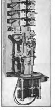
Fig. 50.—Connector switch.
