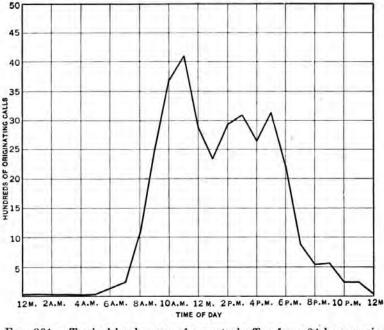
FIG. 301.-Typical load curve of a central office for a 24-hour period.
