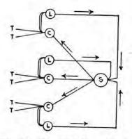
FIG. 13.—Thousand-line exchange (three kinds of junctions).
