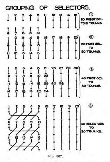
In either case in grouping the lineswitches for the various classes of service, precautions must be taken so that the pay station lines and message rate lines do not have access to the same first selector switches; otherwise, under certain conditions, there would be premature registration of meters on message rate lines, due to the circuit requirements of pre-payment pay station service.
