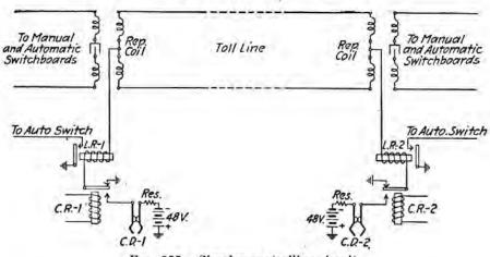
FIG. 255.—Simplex controlling circuit.
