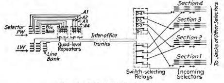
FIG. 74.-Plan of quad-level trunks.
