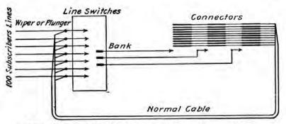
FIG. 9.-One-hundred-line system with Keith lineswitches.
