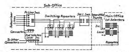
FIG. 33.-Sub-office with switching repeater, 10,000-line system switch on first digit.
