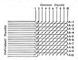
FIG. 125.-Individual trunks with slipped common trunks.
