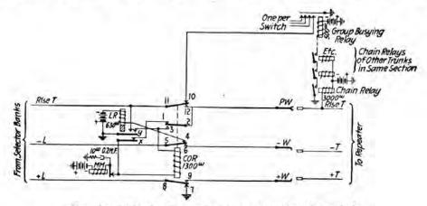
FIG. 80.-Circuit of outgoing rotary secondary lineswitch.
