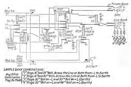
FIG. 83 .- Reverting call switch circuit.
