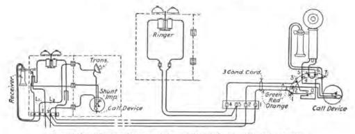
FIG. 148.-Wiring diagram for a wall telephone with an extension.
