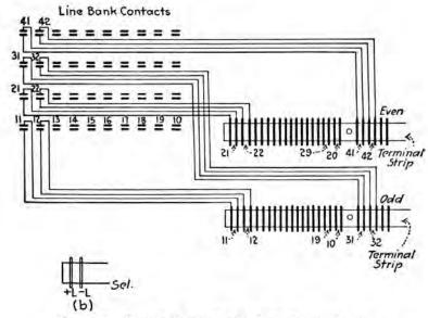
FIG. 102.-Wiring of selector banks to terminal strips.
