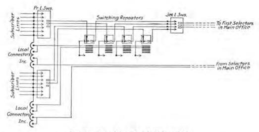
FIG. 32.-Sub-office with switching repeater.
