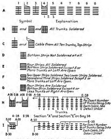
Fig. 107.-Symbols used for terminal assembly solderings.
