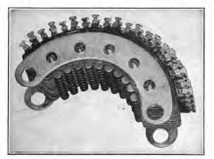
FIG. 55.-Connector-switch bank, unwired.
