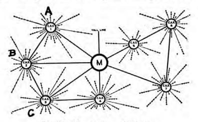
FIG. 270.-Network system of exchanges.
