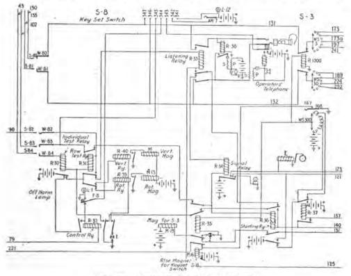
FIG. 179.—Operator's keyset switch circuit.
