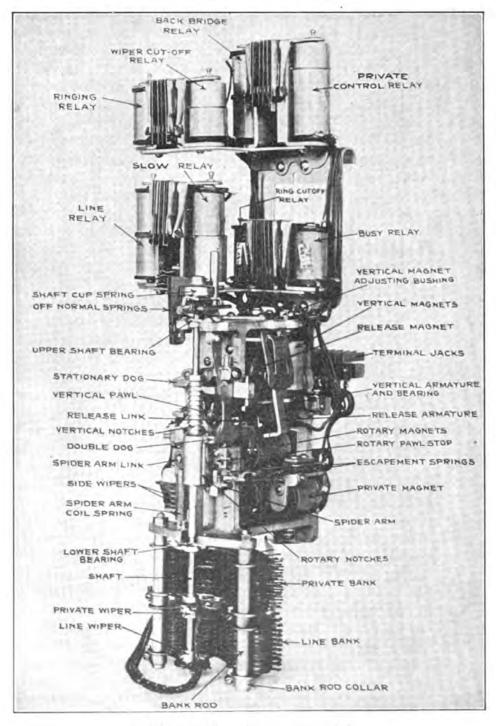
FIG. 42.-Two-wire connector switch.
