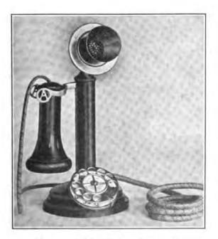
FIG. 30.—Desk telephone instrument.
