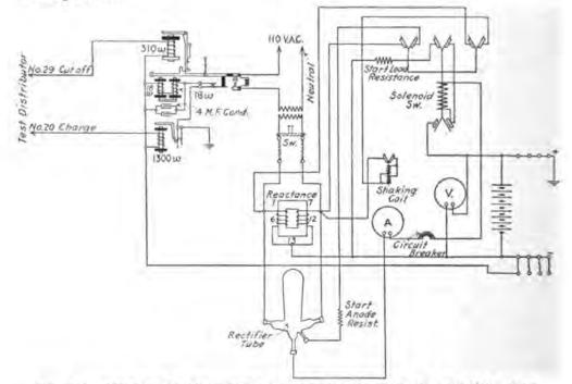
FIG. 244.-Circuits of a Mercury arc rectifier charging outfit for a district station.
