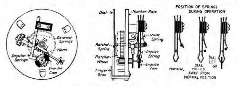
FIG. 32.-Details of calling device.
