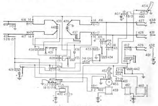
FIG. 213.-Third selector circuit.
