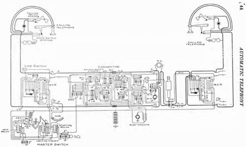
FIG. 41.—Complete circuit from a calling to a called station in a system of 100 lines capacity.
