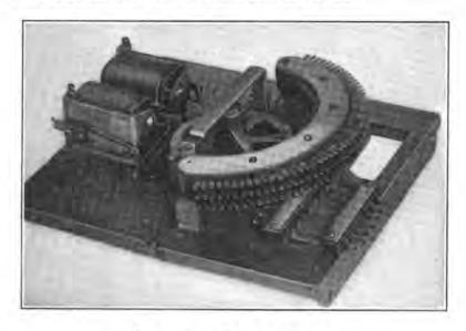
FIG. 90.—Switch bank and wipers.
