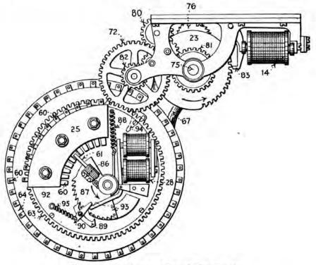
FIG. 133.-Driving gear for cylinder switch.
