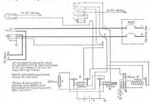
FIG. 254.—Dead number trunk circuit for use in an exchange having metered lines or sub-station coin collectors actuated by "reversing battery" connector switches.
