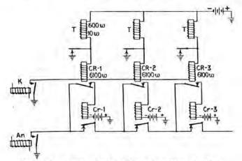
FIG. 118.—Removal of starting relays from circuit.
