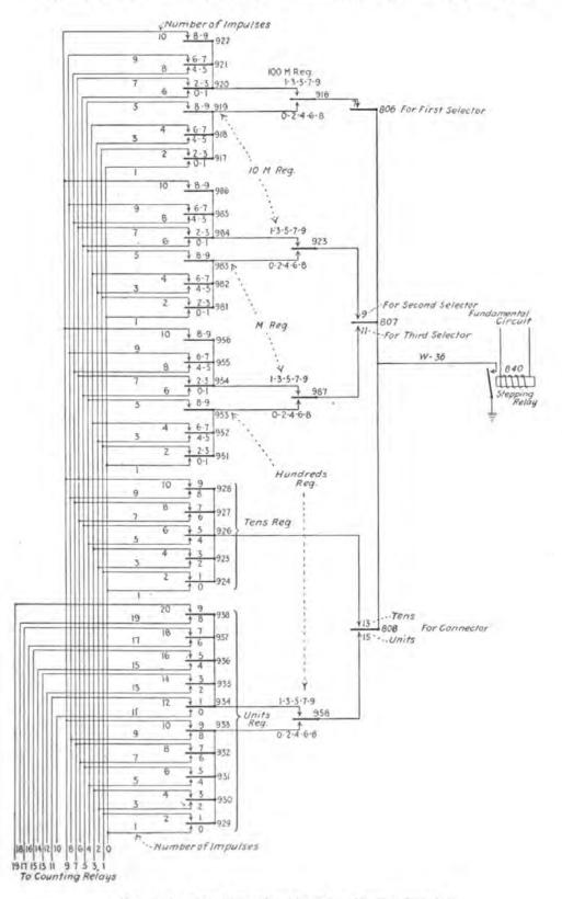
FIG. 226.-Transformation of call number into impulses.
