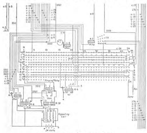
FIG. 144.—Signal transmitter controller circuit.
