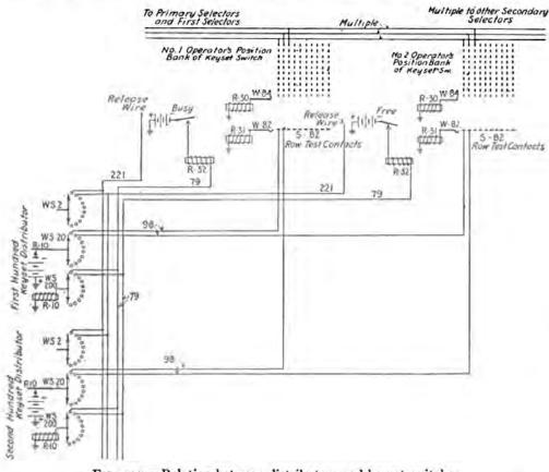
FIG. 177.-Relation between distributors and keyset switches.
