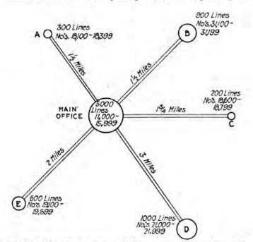
FIG. 269.—Skeleton diagram of a system of three main offices, "Main," B and D, and three district stations A, C, and E.
