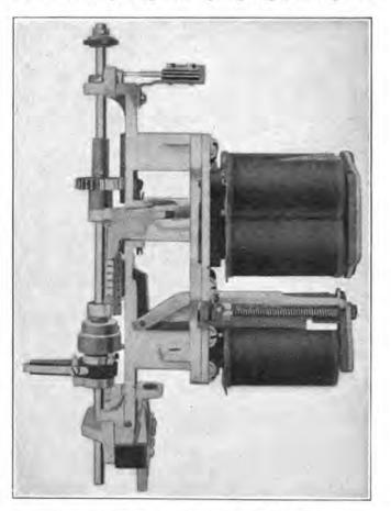
FIG. 192.—Wipers and magnets of switch unit.
