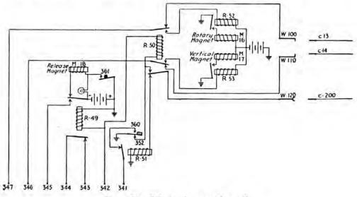
FIG. 186.—Selector for reverting calls.
