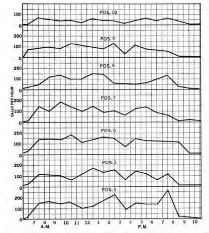
FIG. 151.-Simultaneous load curves of manual switchboard operators' positions.
