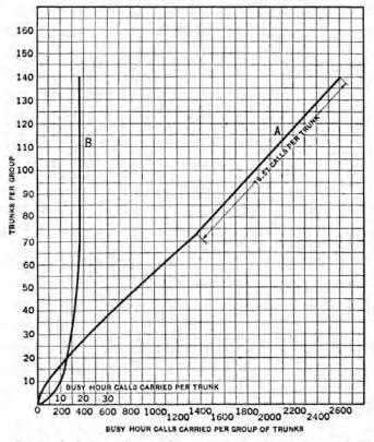
FIG. 262.—Curve A shows call-carrying capacities of trunk groups of various sizes, manual central offices; average trunk holding time of 120 seconds. Curve B shows callcarrying capacity of each trunk in groups of various sizes.
