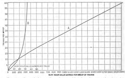
FIG. 263.—Curve A shows call-carrying capacities of trunk groups of various sizes between automatic central offices; average trunk holding time of 83 seconds. Curve Bshows call-carrying capacity of each trunk in groups of various sizes.
