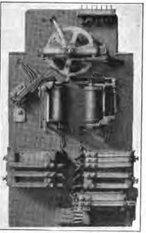
FIG. 92.—Selector switch, magnets and relays.
