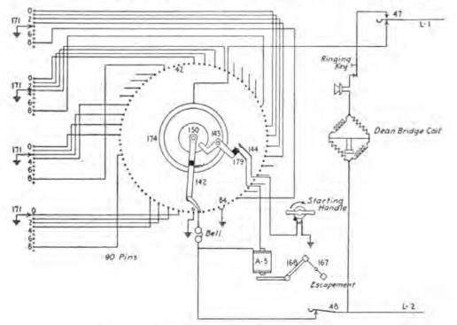
FIG. 137.-Telephone and signal transmitter circuit.
