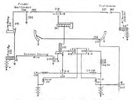
FIG. 225.-Testing circuit of secondary finder and first selector.
