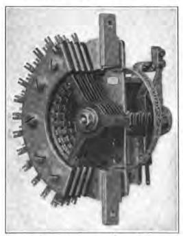
FIG. 102.-Rotary line switch.
