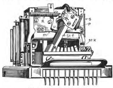
FIG. 105.—Side switch (top view).
