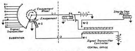
FIG. 138.-Line circuit (telephone to switches).
