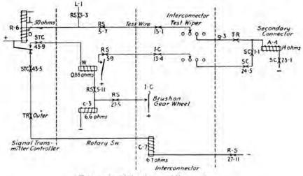
FIG. 148.-Selecting an idle trunk.
