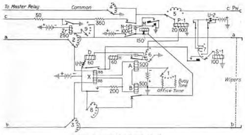
FIG. 109.-First selector circuit.
