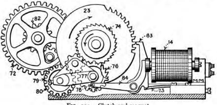
FIG. 134.-Clutch and magnet.
