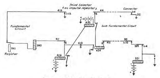
FIG. 227.-Principle of impulse repeater.
