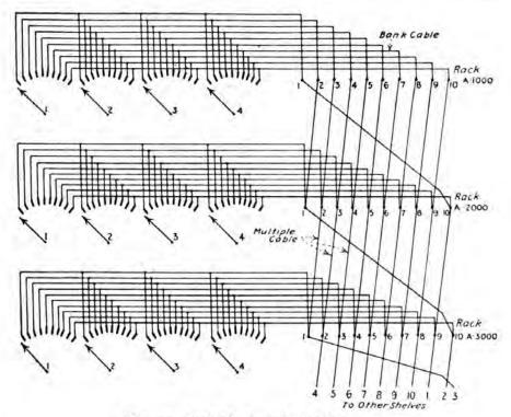
FIG. 14-Bank slip in multiple cable.
