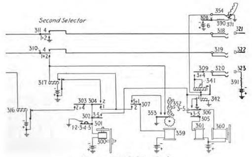
FIG. 212.—Second selector circuit.
