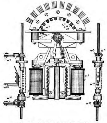
FIG. 194.-Plan-view of 2-motion switch.
