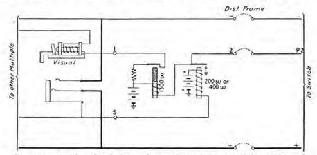
FIG. 233.-Toll-board end of a service trunk to a local automatic switchboard.
