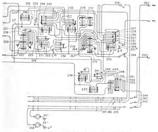
FIG. 96.—Party line connector and frequency selector circuit.
