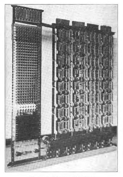
FIG. 201.-Switches mounted on frame.
