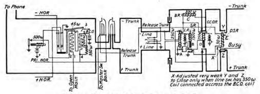
FIG. 74.-Discriminating outgoing trunk circuit.
