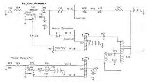
FIG. 219.-Selecting an idle operator.
