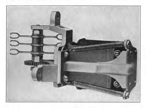
FIG. 189.-Wipers and magnet of rotary switch.
