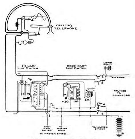
FIG. 60.-Circuit of secondary line switch.
