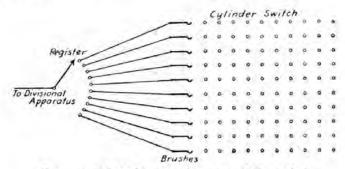
FIG. 132.-Relation of register to cylinder switch.
