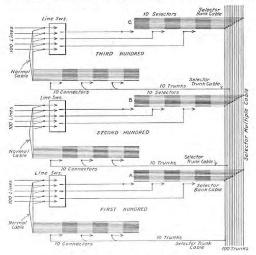
FIG. 22.-One-thousand-line system with line switches.
