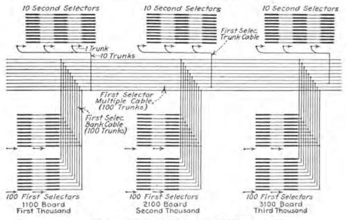
FIG. 9.-Trunking of first selectors by levels.
