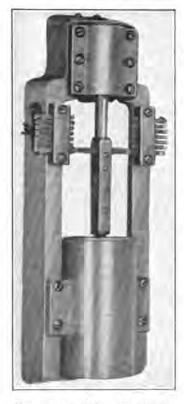
FIG. 241.—Solenoid ringing current interrupter.
