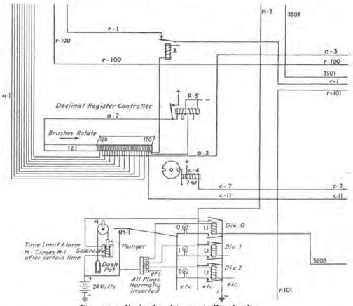
FIG. 140.-Decimal register controller circuit.
