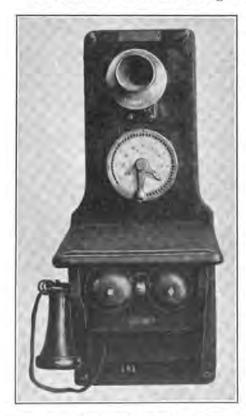
FIG. 88.—Wall telephone with later calling device.
