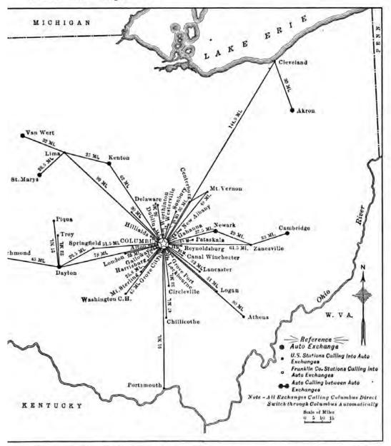
FIG. 237.-Map showing long distance automatic lines centering at Columbus, Ohio.
