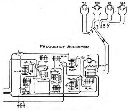
FIG. 62.-Circuit of a frequency selector.
