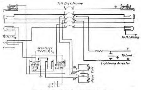
FIG. 229.-A typical toll or rural-line circuit.
