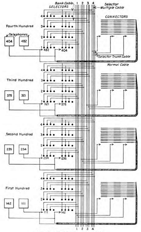
FIG. 6.—Principle of 1000-line exchange.
