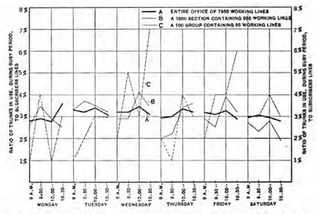
FIG. 261.—Curves showing ratios of trunks in use to susbcribers' lines during the busy hour of each day of a week.
