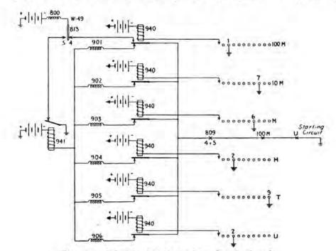
FIG. 222.—Principle of setting registers from keyboard.
