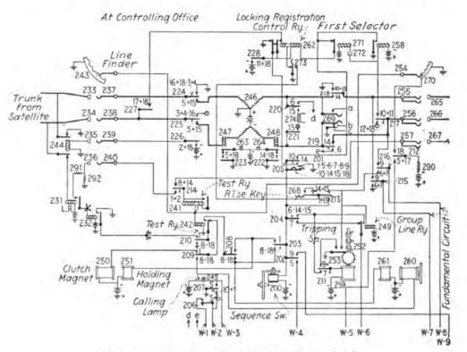
FIG. 211.-Secondary finder and first selector circuit.
