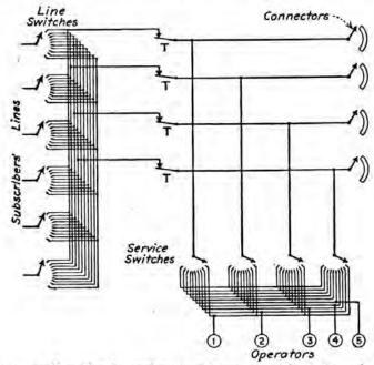
FIG. 119 .- Trunking in semi-automatic system with service switches.
