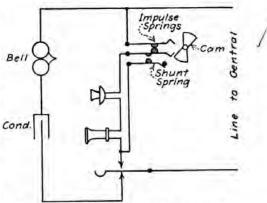
FIG. 33.-Automatic telephone circuit.
