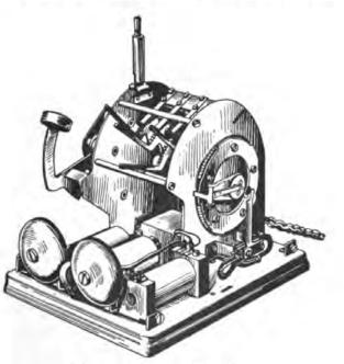
FIG. 101.-Lever calling device.
