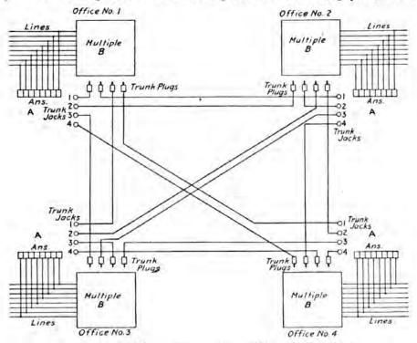
FIG. 3.-Manual inter-office trunking without "A" multiple.
