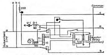
FIG. 106.-Rotary line-switch circuit.
