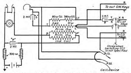
FIG. 258.—Operator's circuit, including calling device, for an information or complaint desk.
