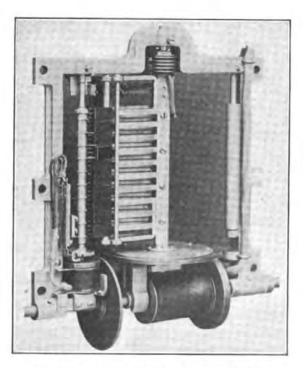
FIG. 203.—Selector brushes and mechanism.
