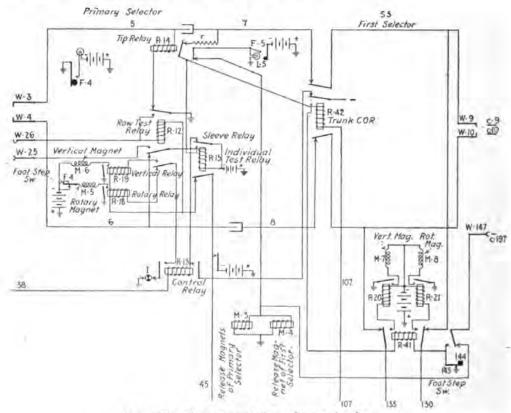
FIG. 178.—Primary and first selector circuits.
