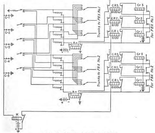
FIG. 116.—Selection of idle trunk to PBX.
