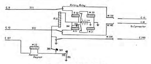
FIG. 182.-Second selector circuit.
