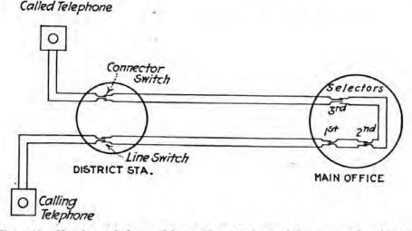
FIG. 268.—Showing switches and inter-office trunks used for a reverting districtstation call.
