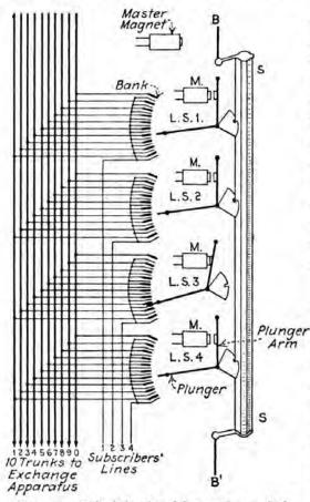
FIG. 20.—Principle of Keith type line switch.
