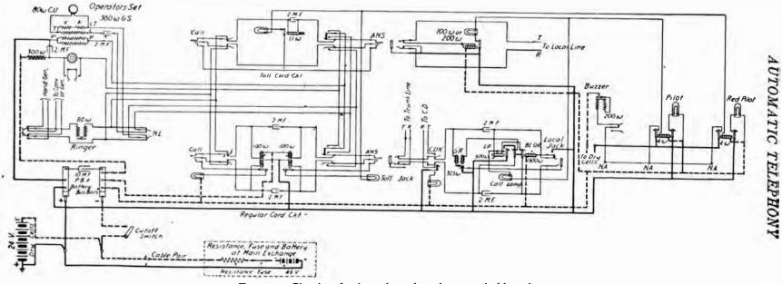
FIG. 73.—Circuits of private branch exchange switchboard.
