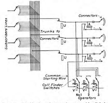
FIG. 122.-Trunking in semi-automatic system with call finders.
