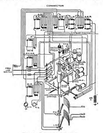
FIG. 50.-Connector-switch circuit.
