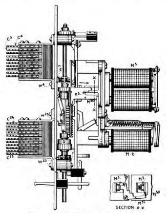
FIG. 193 .- Side view of 2-motion switch.
