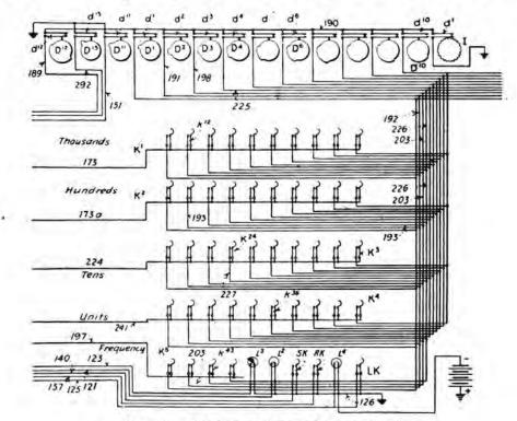
FIG. 181.-Sending machine and keyset circuit.
