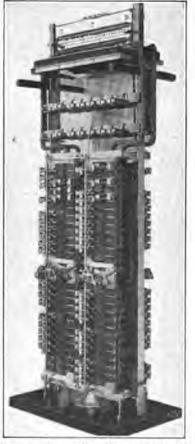
When the plunger enters the bank, spring 1 is pressed against contact 2, thus continuing the release circuit. Contact between springs 5 and 6 continues one side of the line through the first selector and contact between springs 7 and 8 continues the other side of the line. Contact between springs 4 and 3 puts a guarding potential on the proper master switch bank contact.
