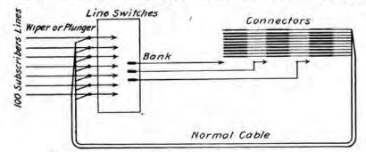
FIG. 21.-One-hundred-line system with line switches.
