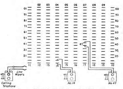
FIG. 4.-Essential principle of connector switch.
