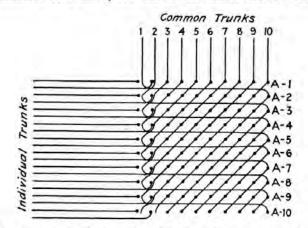
FIG. 17.-Individual trunks with slipped common trunks.
