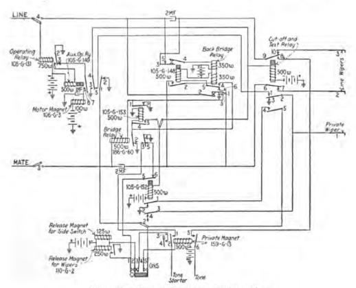
FIG. 170.-Connector circuit at district station.
