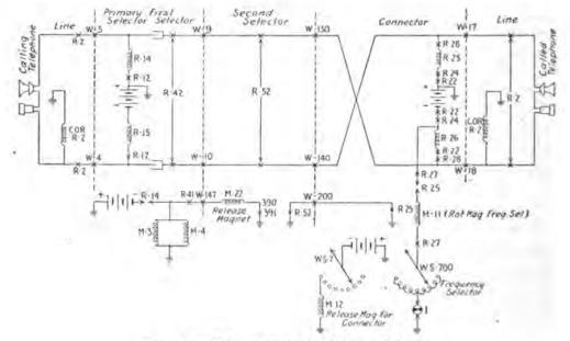
FIG. 185.—Talking connection between stations.
