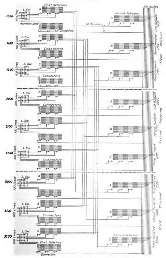
FIG. 23.-Ten-thousand-line exchange with line switches.
