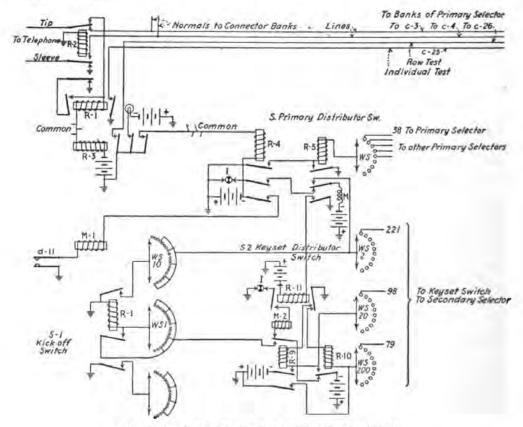
FIG. 176.—Subscriber's line and distributor circuits.
