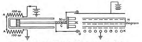
FIG. 158.-Diagram of circuit of Christensen pneumatic selector.
