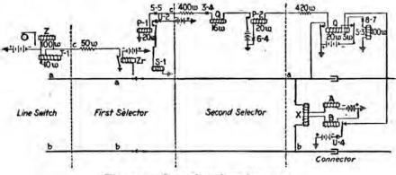
FIG. 112.—Operation of service meter.
