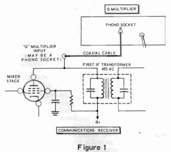
The connection from the mixer plate to the inner lead of the coaxial cable should be as short as possible, and isolated from other receiver circuits. If shielded wire is used for the connection between the coaxial cable and the mixer plate, the primary winding of the first IF transformer should be retuned. (Retune the transformer before attaching the Q Multiplier to the receiver.)
