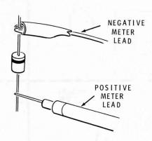
Proceed to the following chart and connect the ohmmeter leads to the component as indicated in the columns titled "Connect Positive Lead To," and "Connect Negative Lead To." The indicated meter reading in the last column is only a nominal reading. Your meter may read slightly different.
