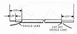
TAKING CARE NOT TO CUT THE SHIELD LEAD, REMOVE THE OUTER INSULATION.
