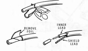
REMOVE THE FOIL AND REMOVE 1/4" OF INSULATION FROM THE END OF THE INNER LEAD. **Detail 4-7A**
