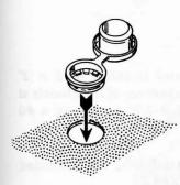
POSITION THE SMALL PORTION OF THE GROMMET INTO THE SHASSIS HOLE.
