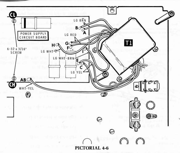
Connect the wires coming from BO#6 of the harness to the power supply circuit board as follows:
