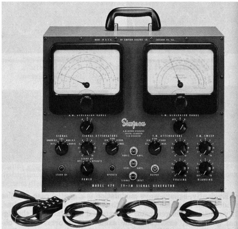
Fig. 3-17. Typical fm/am generator.
