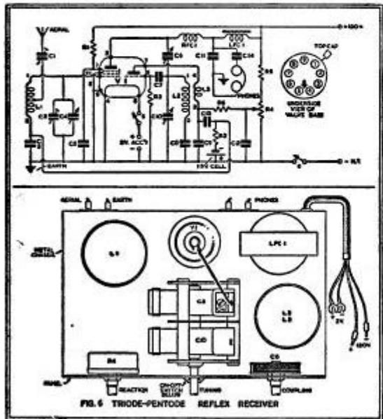
to-easy, and any method by which parts could be dispensed with was considered a major advantage. In a reflex receiver, one valve is made to perform the duty of two or more by shunting the signal round the circuit, by-passing any unwanted portion and returning it to its point of entry for yet further amplification. This system is not to be confused with the more orthodox process of using, perhaps, a double triode in a straight circuit one half as a detector and the other half as an amplifier.
