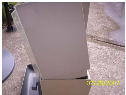
Once all three candy bins have been inserted into the top of the main assembly you place the top security cover onto the machine. Make sure that the "vendstar" logo is at the front, or else it won't attach.
