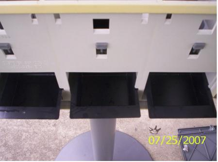
Once you place the money bins all the way into the machine, you place the back of the machine into the unit from the top until it closes on the bottom. You use the vending style key to lock the back door and protect your monetary gains.
