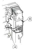
4 Tilt the keypad assembly outwards, unplug the display loom, and then lift upwards to unhook the lower retaining lugs from the spine – steps C D and E
