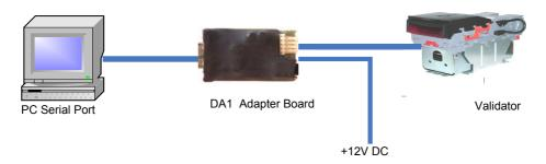
Figure 1 - Connecting DA1 to a NV9 and PC for upgrading
