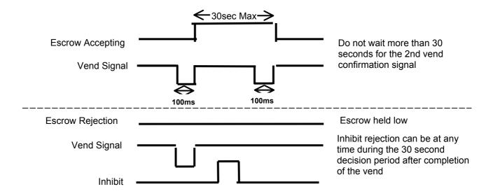
Figure 19 - Escrow Timing Diagram for Parallel Vends
