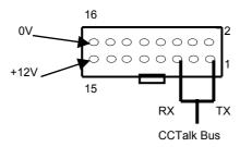
Figure 7 - CCTalk Connection Pins on the NV9
