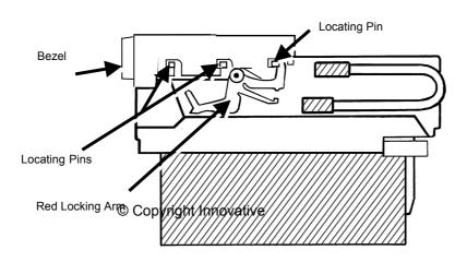
Figure 10 - Bezel and Validator Removal
