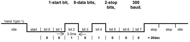
Figure- 5 Typical Serial Output: Transmission of the value 20 (decimal), Note not recognized
