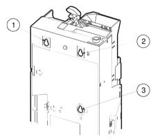
The vending machine is generally fitted with three screws in matching positions. Alternatively, there may be two location studs and one screw, or a similar arrangement.
