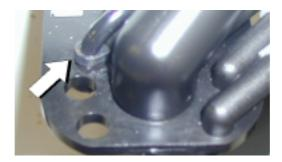
• The material of the hose from the pump to the flowmeter has been changed into a softer material in order to reduce the vibrations in relation with water dosing. This should prevent that less espresso water than the actual setting is dosed.
