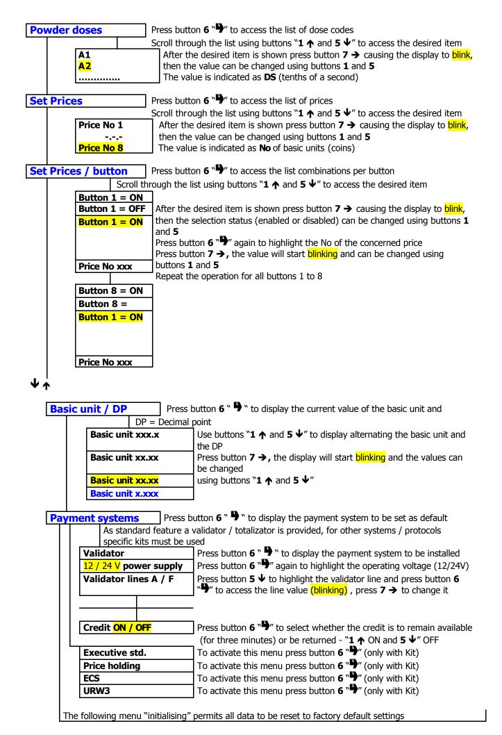
It must be used in the event of data (RAM) errors or of replacing the EPROM: After initialising all data that were changed from the default settings must be reprogrammed.
