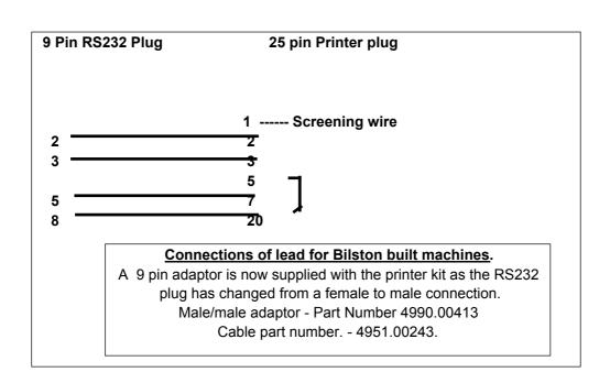
By using the <u>Sankey printer</u> and changing the <u>Baud rate,data</u> <u>bits and parity</u> it is possible with the <u>Sankey printer lead</u> to print off the statistics from the Zanussi range of equipment. Machines tested: Zenith,Brio,Brio250,Granmatti,Colibri,Starfood,Smart,Spring
