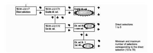
These direct selection buttons can also be set to vend any 'Virtual Selections' that are set-up on the machine (see instruction below). Proceed as per instruction above until the \*. When you press E and the  $1^{st}$  '00' flashes you then enter the 'Virtual Selection' number (70 – 79). This will automatically enter the same 'Virtual Selection' number into the  $2^{nd}$  '00'. The direct selection button is now set to vend the two products set-up in the 'Virtual Selection' menu.
