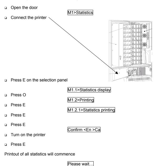
When printout has ended, disconnect printer and close machine door
